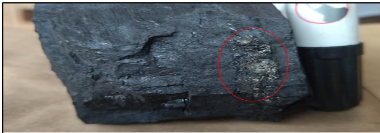
Figure 4.15: Hand specimen showing a dull coal with framboidal pyrite grain.
