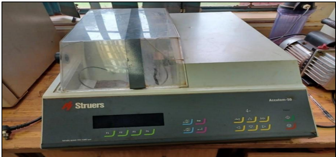
Figure 3.11 A Struers Accutom-50 cutting machine for cutting the samples for thin section preparation
