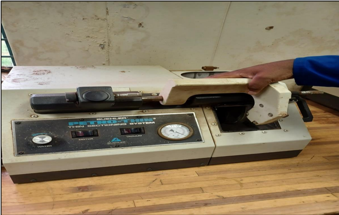
Figure 3.10: A Bushler petro-thin sectioning system for cutting during the thin section preparation
