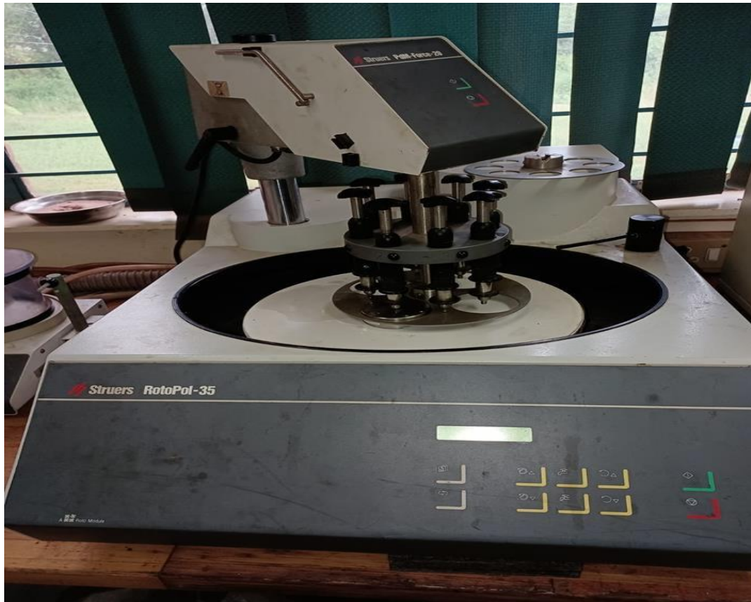
Figure 3.12: The RotoPol-35 polishing machine used during the thin section preparation
