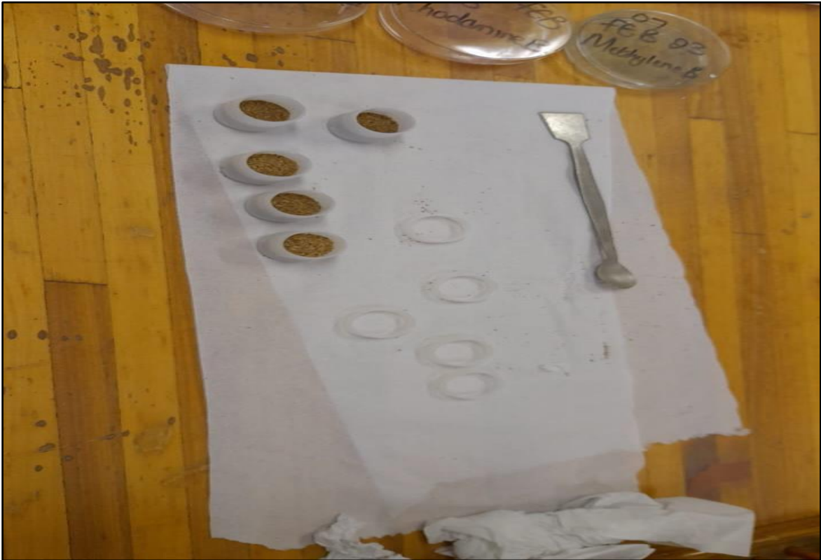
Figure 3.15: Pouring of Sediment samples into the PVC cup during the XRF sample preparation
