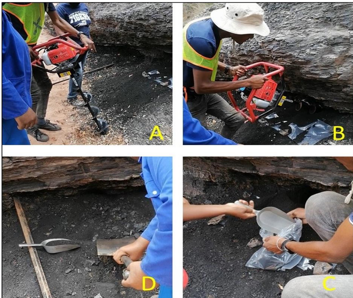
Figure 3.4: Coal sampling: (A) earth auger, (B) drilling along the dip direction, (C) sample collection, (D), Rehabilitation.
