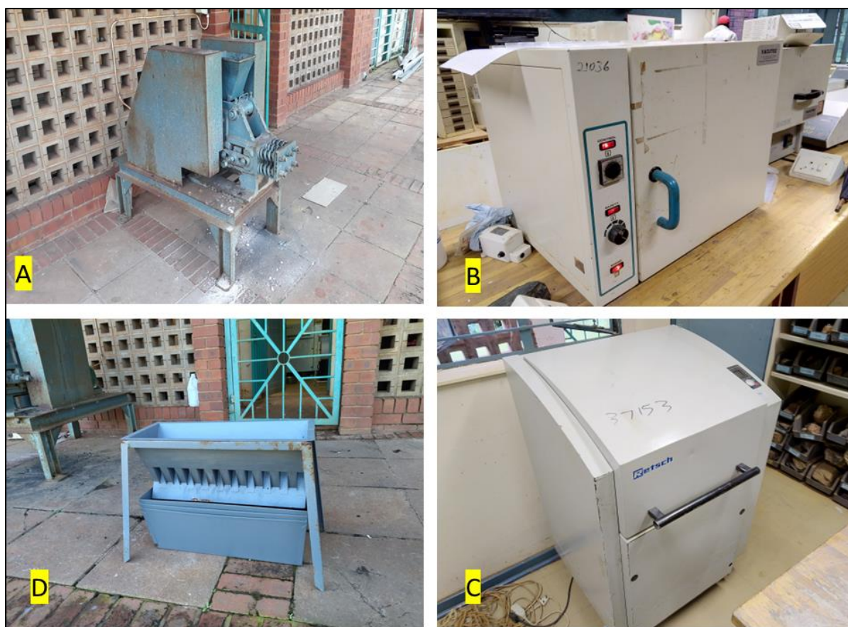
Figure 3.6: Laboratory equipment: (A) Jaw crusher, (B) Drying oven, (C) Milling machine, (D) Riffle splitter.
