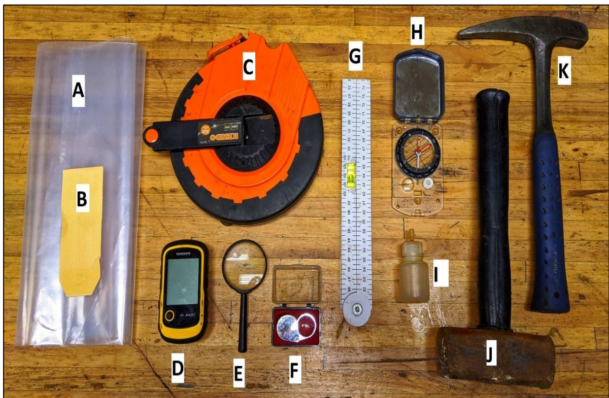
Figure 3:3: Geological field mapping tools: (A) sample bags, (B) Tags, (C) 50 m measuring tape, (D) Garmin eTrex 10 GPS, (E) magnifying glass, (F) jeweller's loupe hand lens, (G) clino ruler, (H) Brunton Compass, (I) Diluted hydrochloric acid, (J) sledgehammer, (K) geological hammer.
