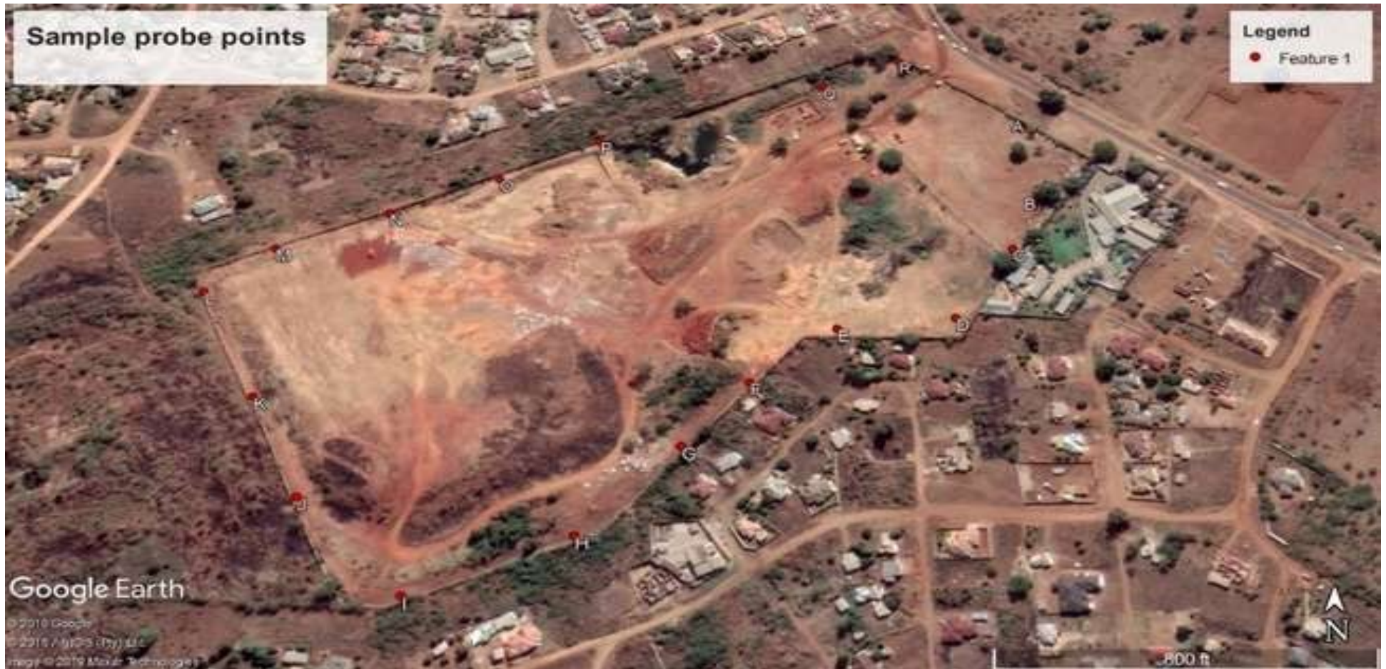
Figure 3.2: Aerial view of the landfill site showing the different points the LFG monitoring probes were installed at the boundary of the landfill. Note: Point A–R shows the points where the monitoring probes were installed in the landfill.
