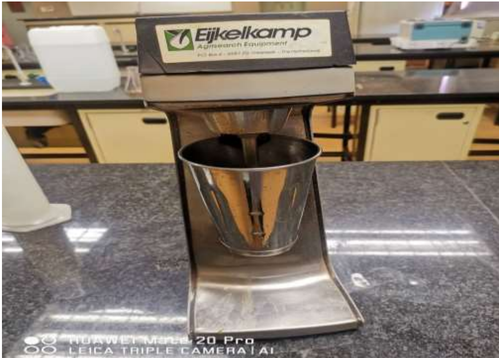
Figure 0-6: Sediment Slurry Preparation Using a Reciprocating Shaker
