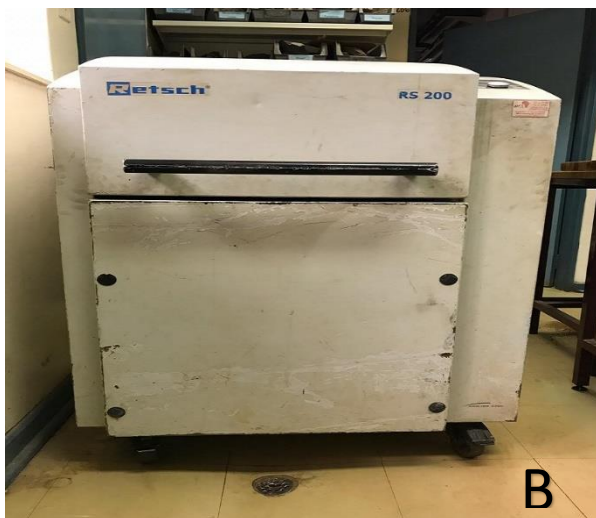
Figure 3.5: Laboratory equipment: A) Vacutec drying oven; and B) Restsch RS 200 milling machine used to prepare coal samples.
