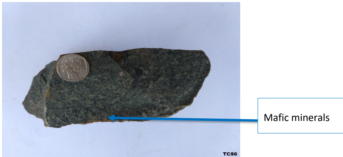
Plate 4.10: Dolerite specimen showing mafic minerals.
