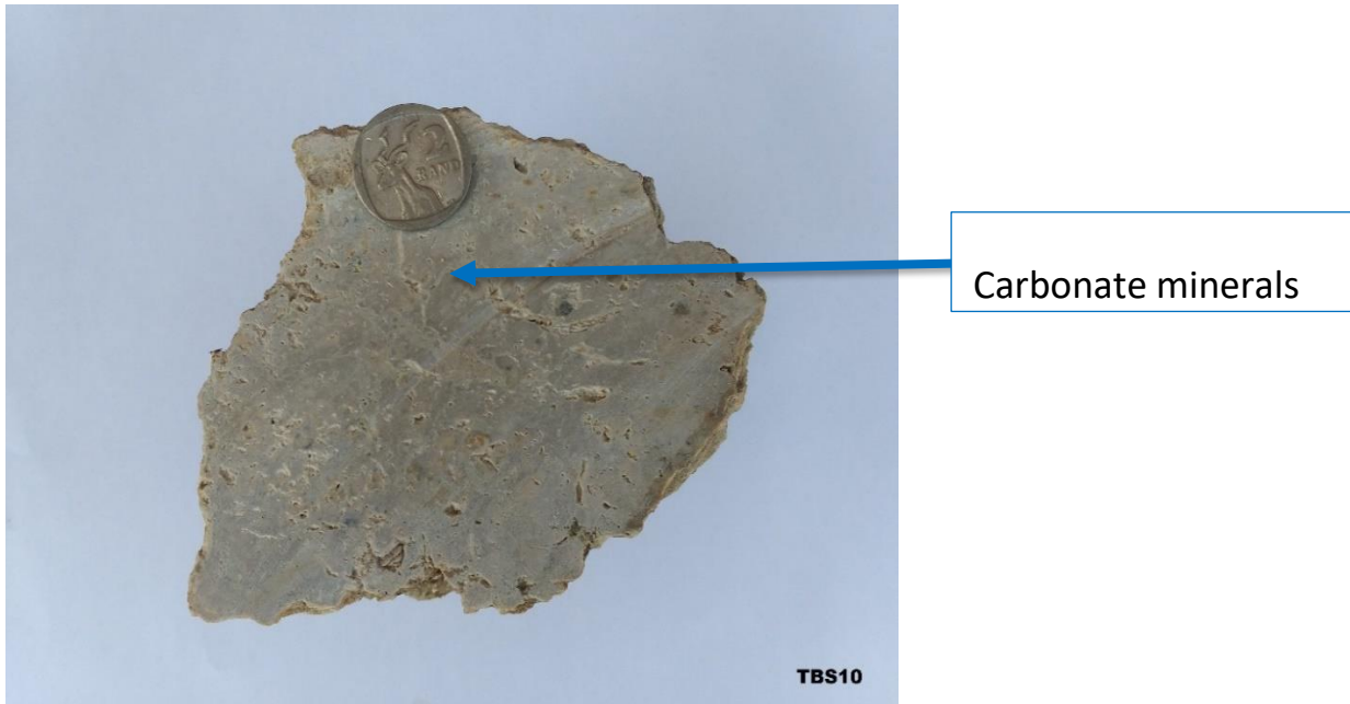
Plate 4.3: Calcrete specimen containing carbonate minerals with very fine texture.
