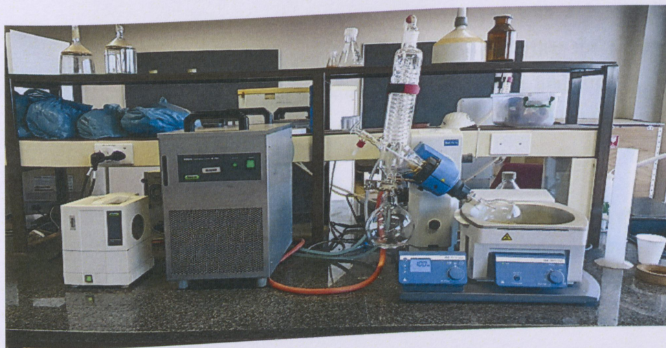
Figure 3.2.1: Büchi Rotavapor ® RII (with distillation chiller and vacuum pump) used for evaporating organic extracts.
