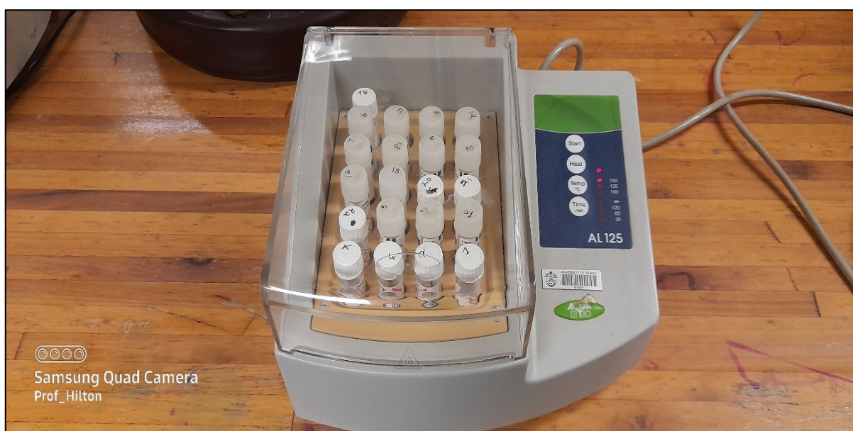
Figure 3.3: Samples in thermoreactor for COD analysis.
