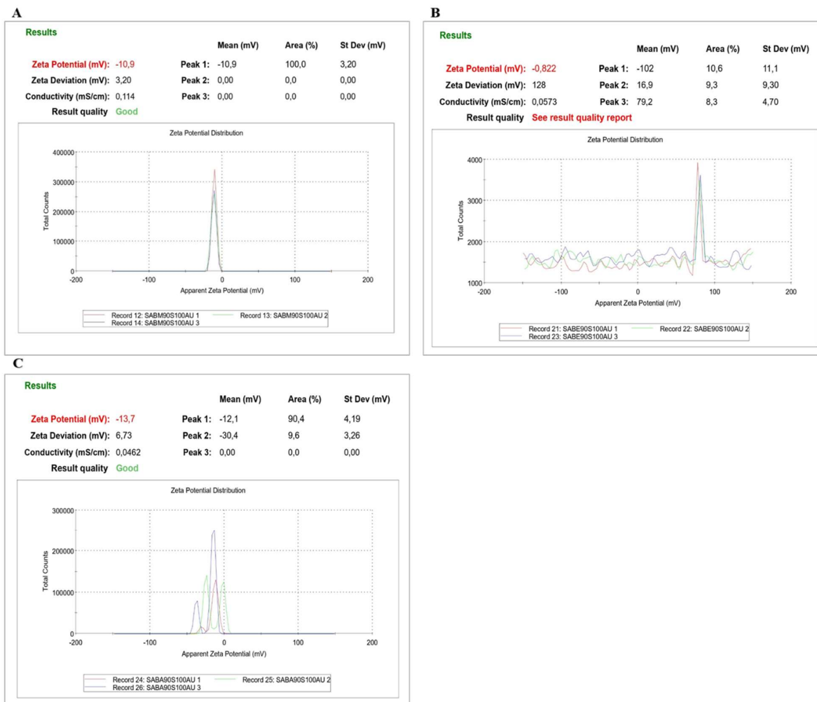
Figure 4.10: Zeta potential (ZP) stability analysis of the produced SA-AuNPs. A= SABM-AU (bark methanol conjugated AuNPs), B= SABE-AU (bark ethanol conjugated AuNP), and C= SABA-AU (bark acetone conjugated AuNP). Each sample was run in triplicates.
