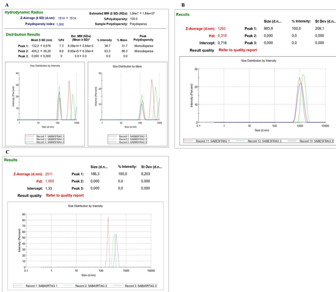
Figure 4.7: Dynamic light scattering (DLS) analysis for particle size of synthesised SA-AgNPs. A= SABM-AG (bark methanol conjugated AgNPs), B= SABE-AG (bark ethanol conjugated AgNP), and C= SABA-AG (bark acetone conjugated AgNP). Each sample underwent three runs.
