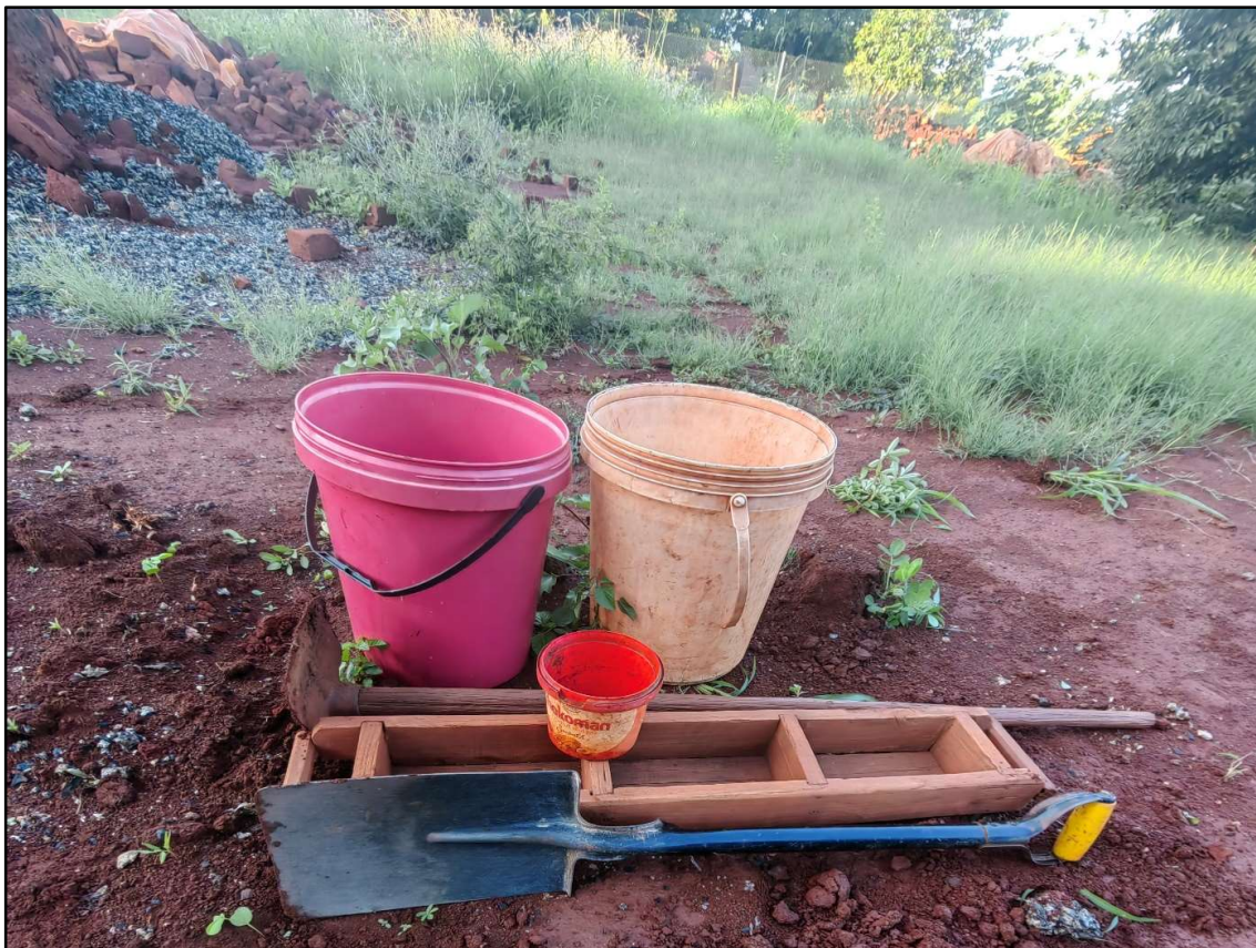
Figure 3. 7: Equipment and tools used for brick production: mould, shovel, water, and measuring container.
