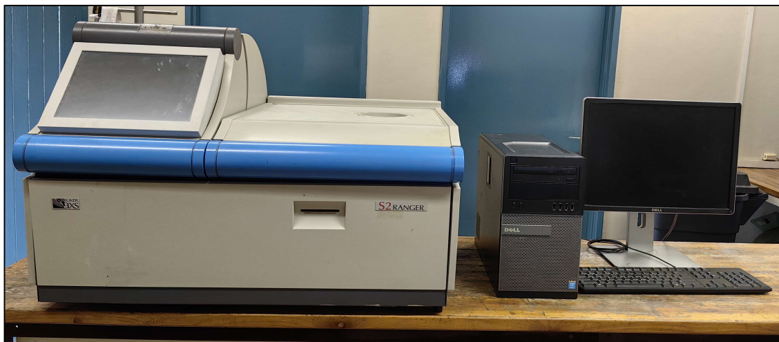
Figure 3. 15: Photograph of S2 Ranger XRF equipment used for metals analysis.
