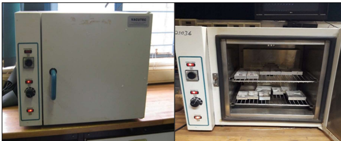
Figure 3. 12: Bench Vacute laboratory oven used for drying samples.
