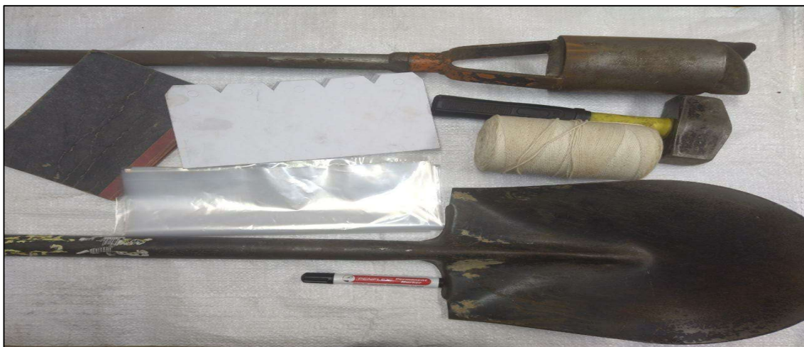
Figure 3. 2: Equipment and tools used for fieldwork: hand auger, shovel, notebook, pen, marker, sampling tags, sampling bags, string and hammer.
