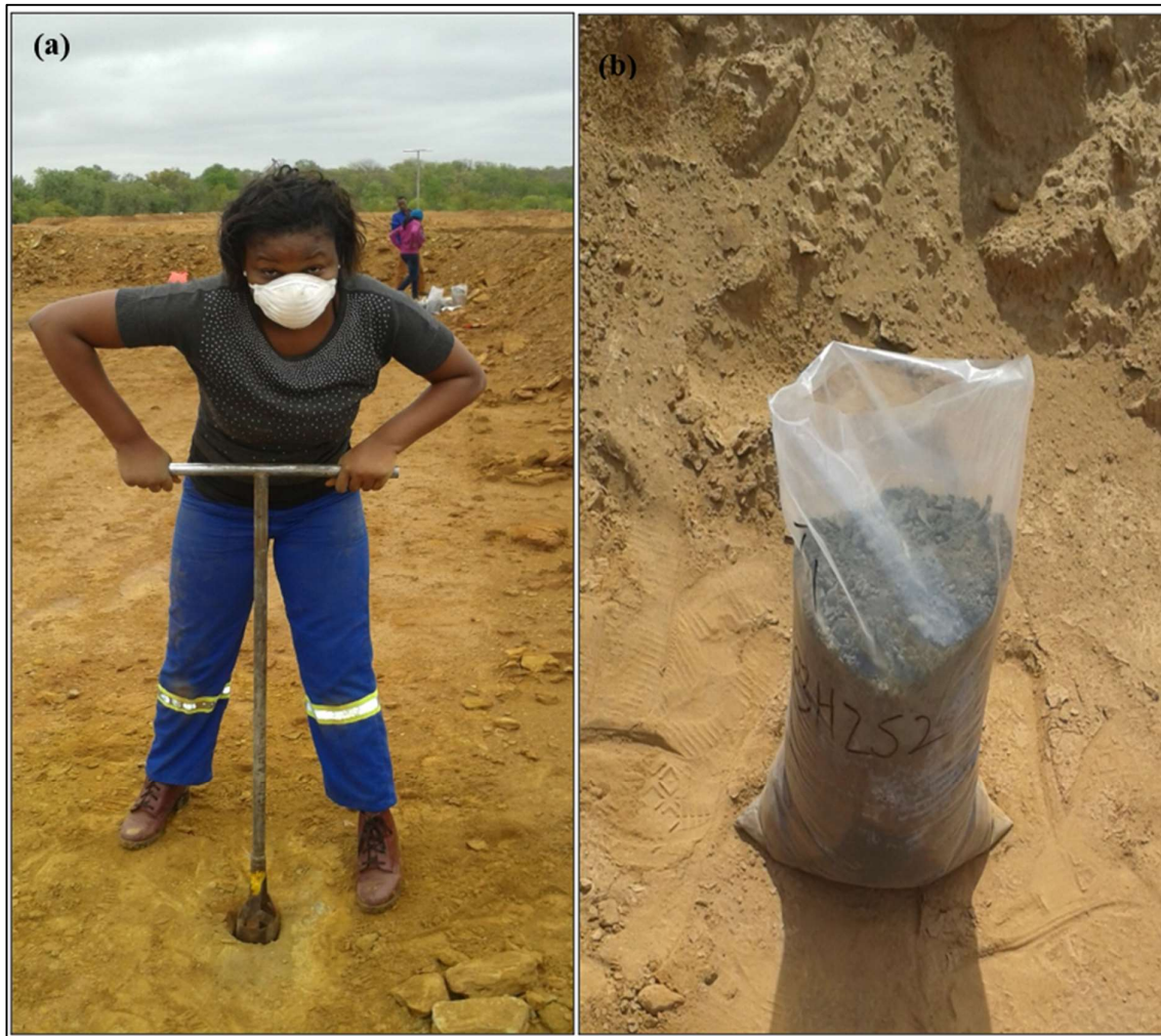
Figure 3. 6: Tailings sample collection: (a) hand auger drilling; (b) collected sample in labeled sample bag.
