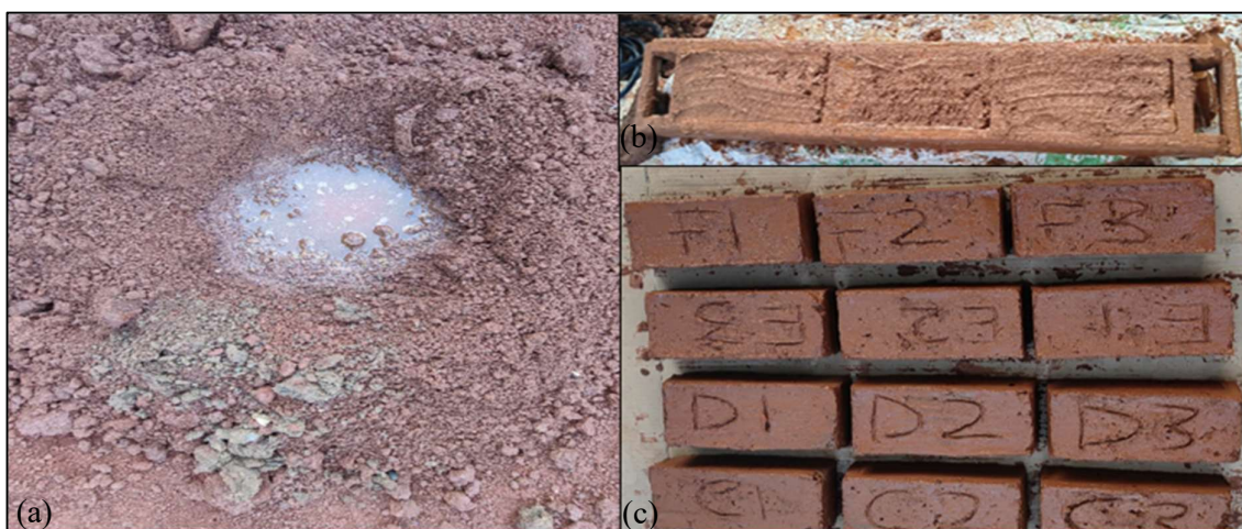
Figure 3. 8: Photograph illustrating brick making process: (a) soil, tailings, and water; (b) brick mould with mortar; and (c) bricks.
