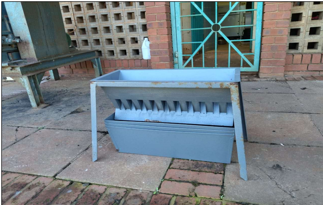
Figure 3. 11: Riffle splitter used to homogenize the samples.
