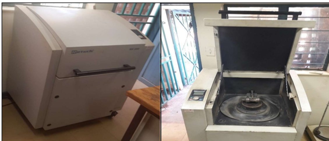
Figure 3. 13: Retsch model RS 200 milling machine used for milling samples.
