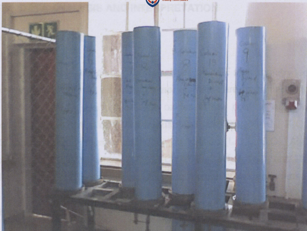
Figure 11. The column leaching experimental set up for phase 2.
