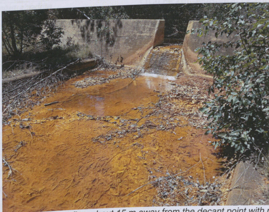
Figure 7. Acid Mine Drainage decants from an old abandoned flooded coal mine in the Witbank Coal field (CGS, 2013).
