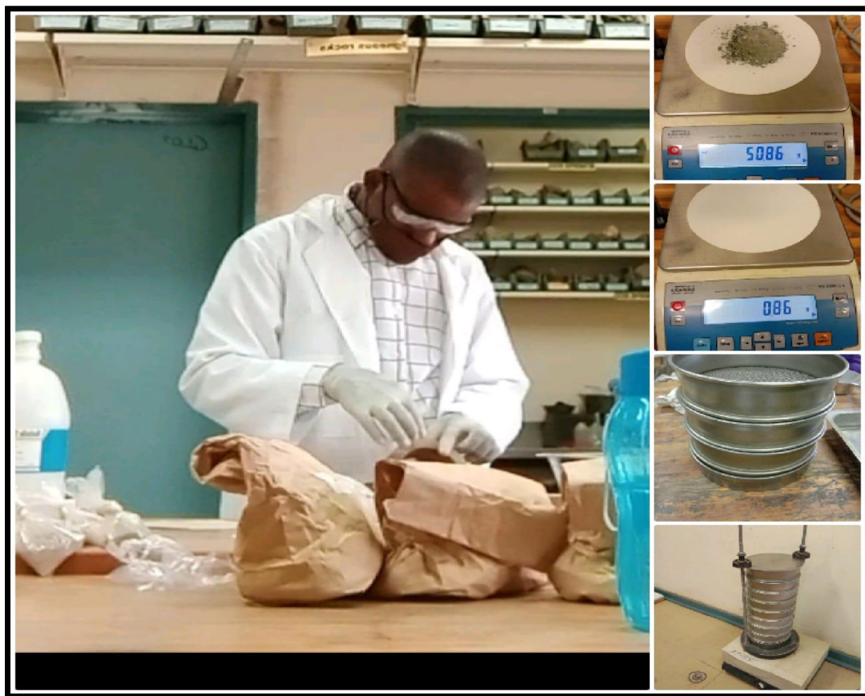
Figure 3.10: The procedure of sieving soil samples.
