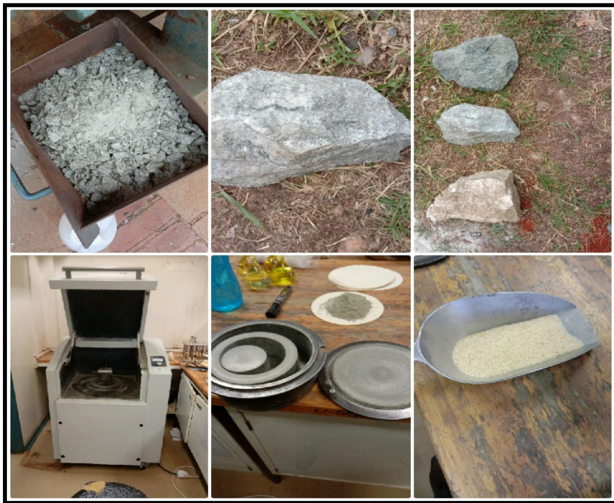
Figure 3.11: The process of crushing and milling rock samples.
