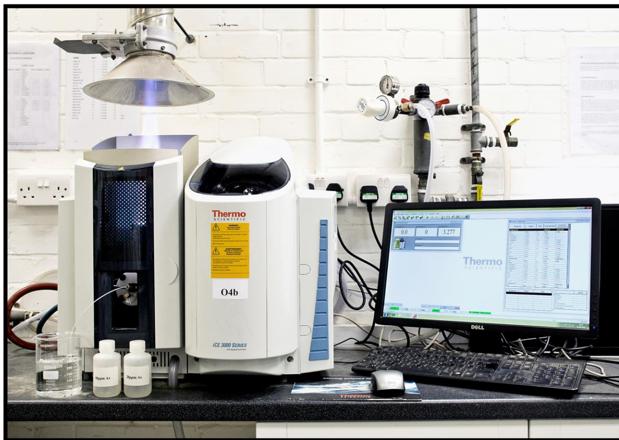
Figure 3.14: Analysis of the soil sample using AAS (Silvia et al., 2004).
