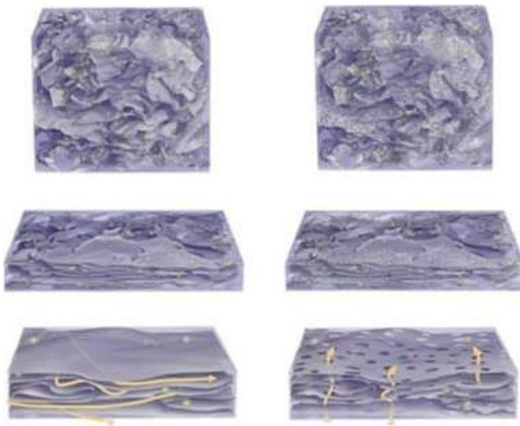
Figure 4: Schematic illustration of graphene and holey graphene forms. Initial 3D macroporous (a) graphene foam and (b) holey graphene foam. Compressed films of the (c) graphene foam and (d) holey graphene foam. Close-up views of (e) graphene and (f) holey graphene films. The arrows highlight the ion transport pathway (Xu, Lin, et al. , 2015).
