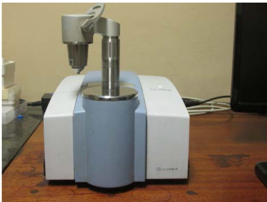
Figure 3.4 Fourier transform infrared (FTIR) spectroscopy instrument. Photograph taken by C. Anokwuru
