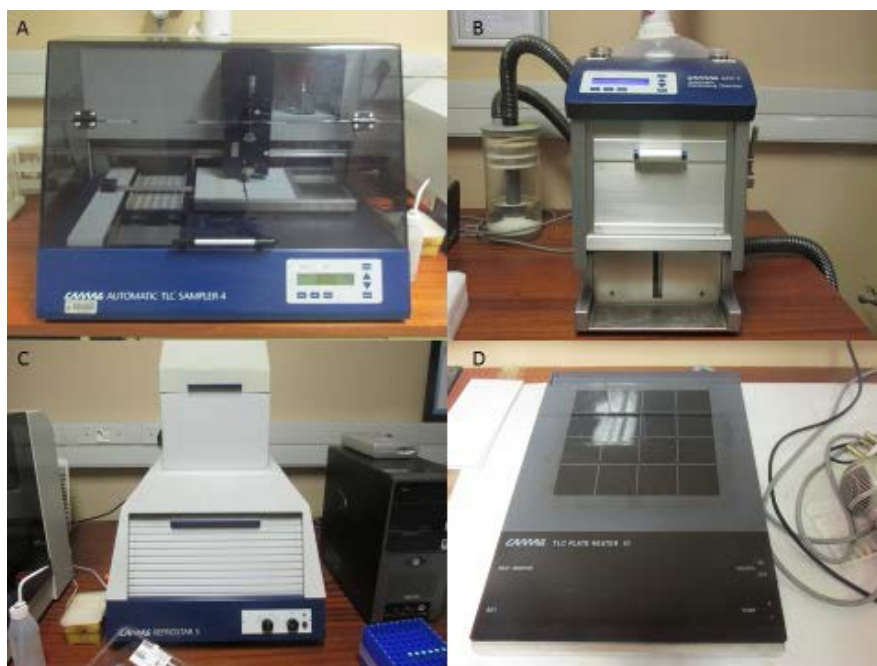
Figure 4.2 High performance thin layer chromatography system (CAMAG) consisting of A) automatic sampler, B) automatic developing chamber, C) reprinter (scanner), D) plate heater. Photograph taken by C. Anokwuru
