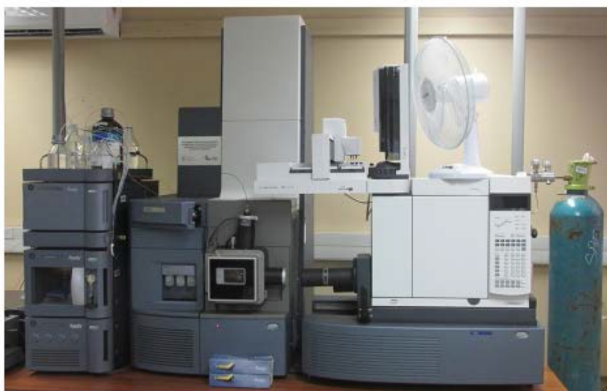
Figure 3.2 UPLC-QToF-PDA/MS instrument used for analysis of the semi-purified and purified compounds. Photograph taken by C. Anokwuru
