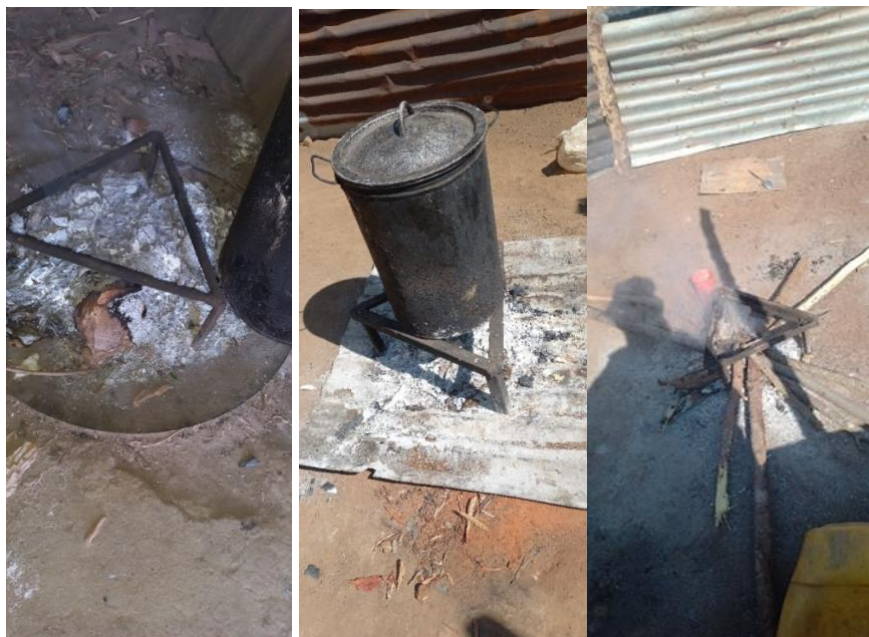
Figure 4.1: Three-legged iron stove used to cook and boil water by the households.
