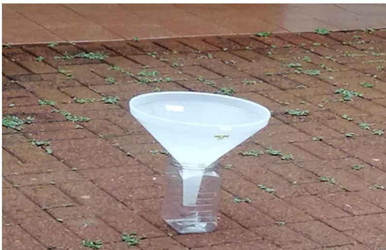
Figure 3.3: A schematic picture of a bottle and a funnel that were used to collect rainwater samples
