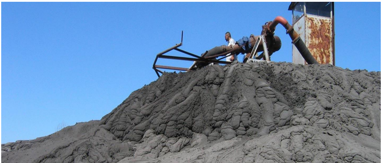
Figure 2.1: Ash pumped as slurry into ash dams (Chemin, 2014).
