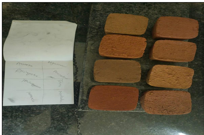
Figure 3. 5: Clay blocks in sequence before furnace firing
