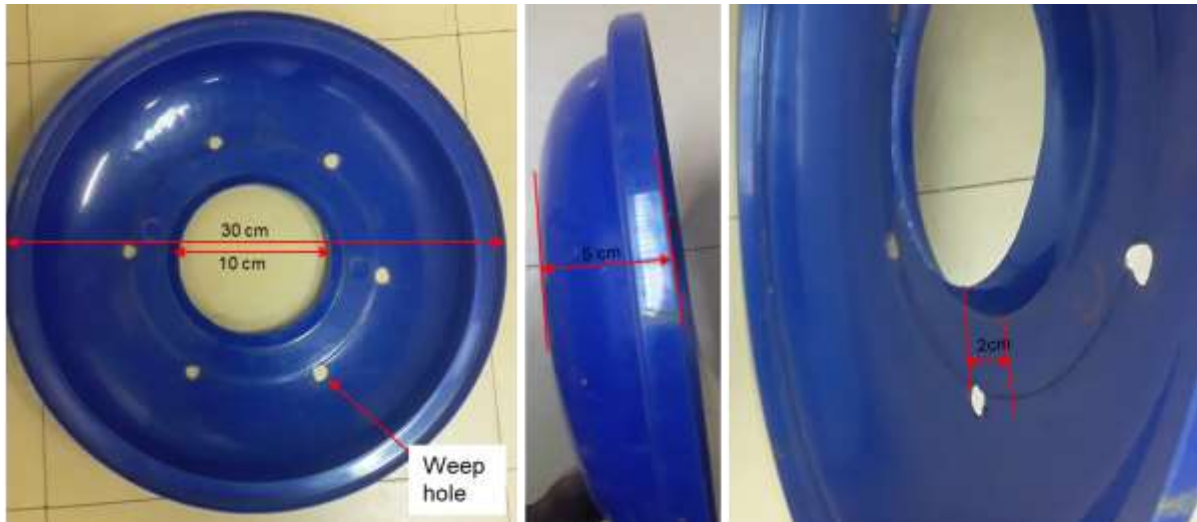
Figure 0.2: Splash Cup Design (adapted from Morgan, 1981)
