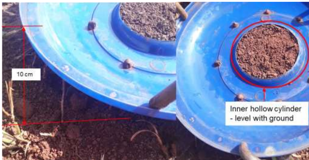
Figure 0.4: Splash Cup Set-up in the Field
