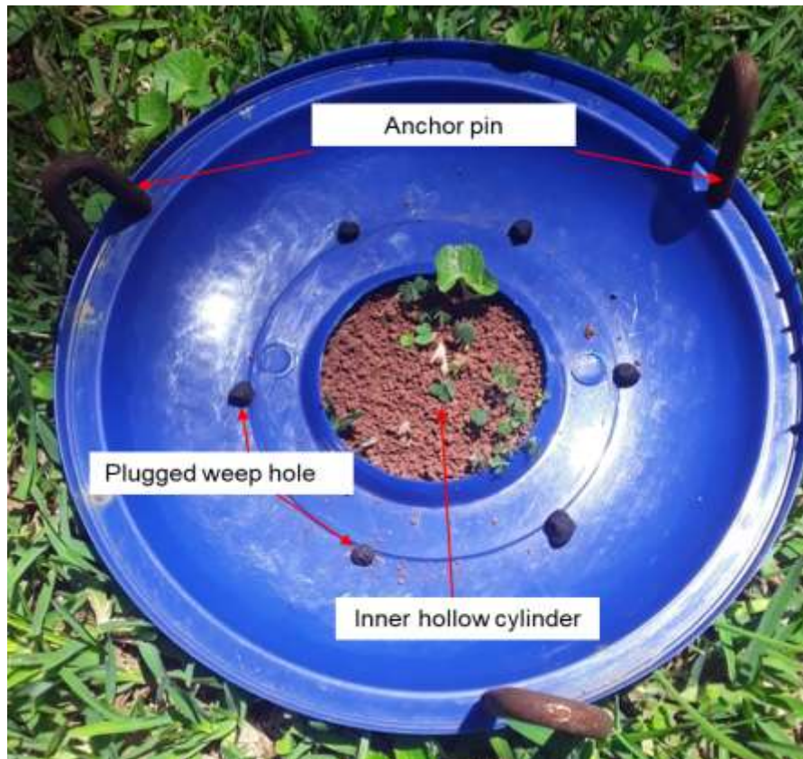
Figure 0.3: Splash Cup Set up Demonstration
