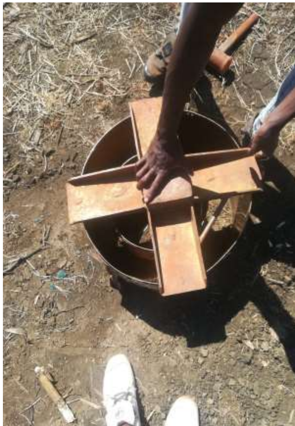
Figure 4a: double ring infiltrometer
