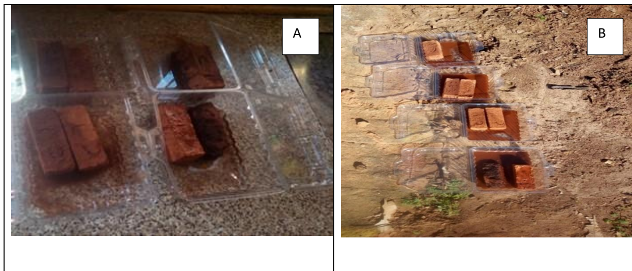
Figure 5.4: Efflorescence of clay bricks, A-submerged bricks, B-exposed modified bricks
