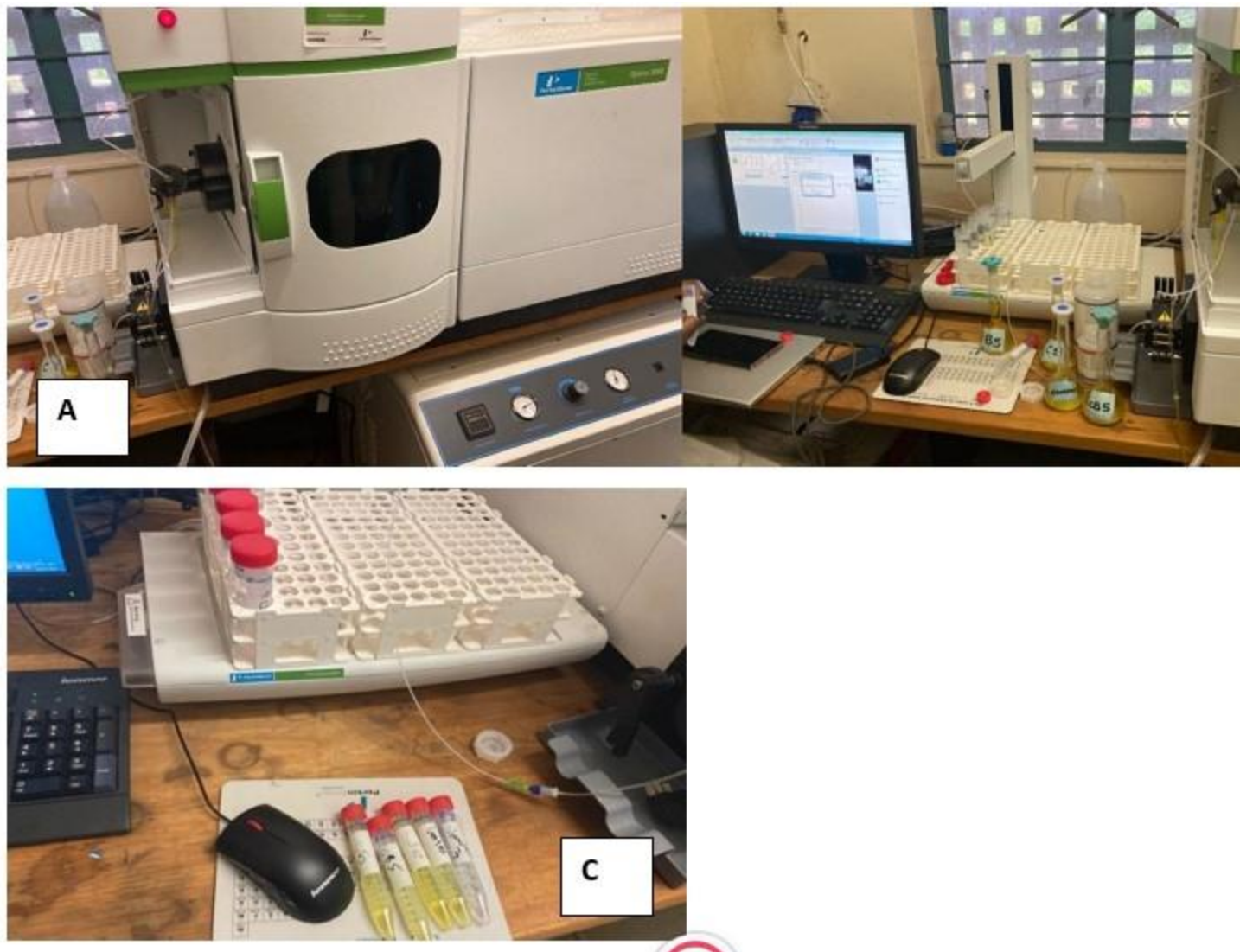
Figure 3.4: Metal Analysis. A -ICP-OES. B -Preparation of samples and C -analyzed samples.
