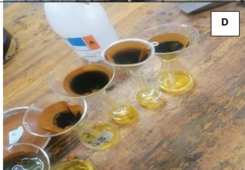
Figure 3.3: Acid digestion of clay. A -preparation of clay, hydrochloric acid and nitric acid B -Hot stove digestion, C -Filtering of decomposed samples and D - Filtered sample ready for ICP-OES.
