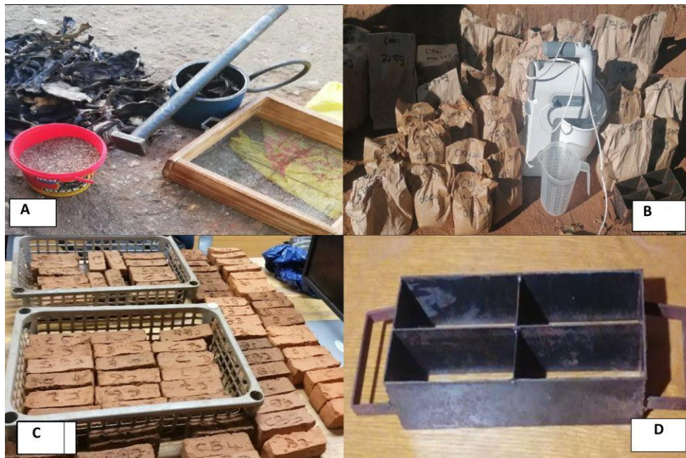
Figure 3.2: Process of making modified clay bricks. A -Banana Biomass; B -Brick making process; C -sundried bricks and (D) miniture bow box mould.
