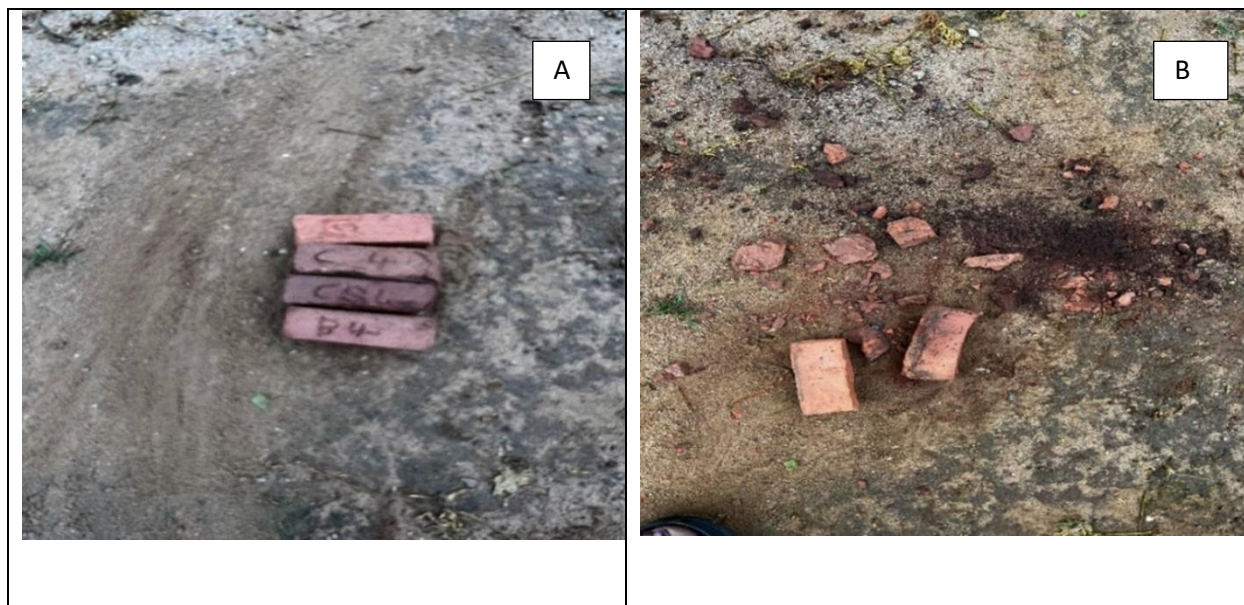
Figure 5.3: Impact test of the bricks (A) before the impact and (B) after the impact
