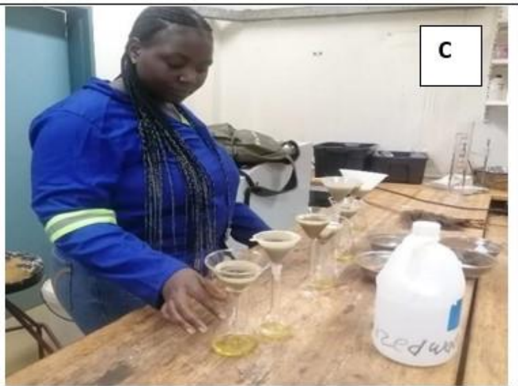
Figure 3.3: Acid digestion of clay. A -preparation of clay, hydrochloric acid and nitric acid B -Hot stove digestion, C -Filtering of decomposed samples and D - Filtered sample ready for ICP-OES.
