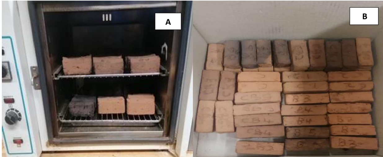
Figure 5.2: Color of the bricks, A -firing of modified clay brick, B -overheated modified bricks
