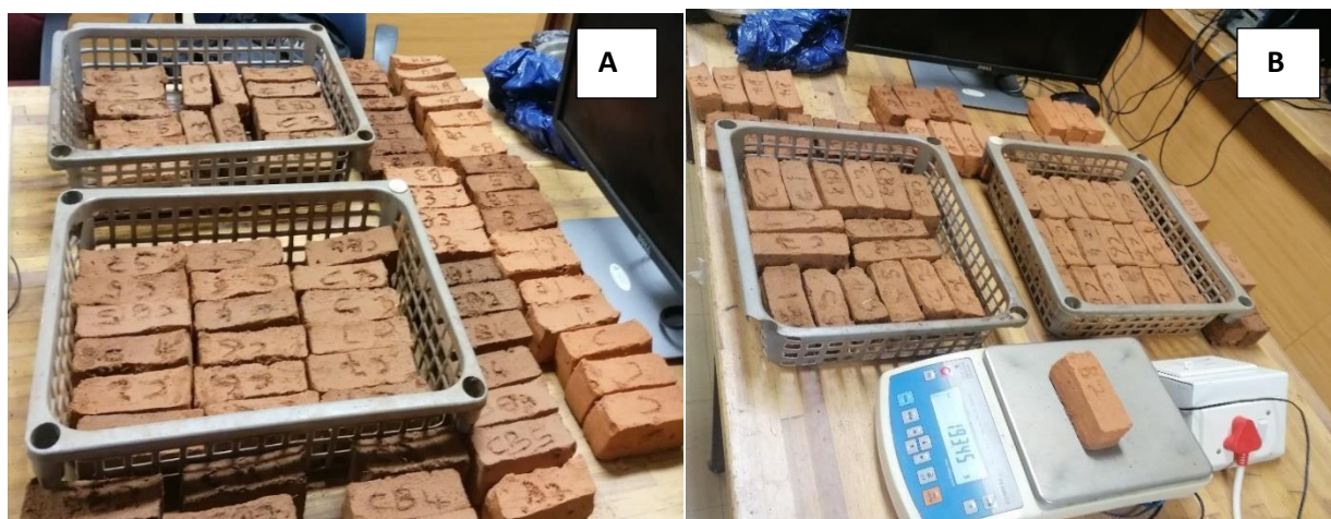
Figure 5.6: Wrappage test of the bricks. A -fired modified bricks, B -level of the modified bricks.
