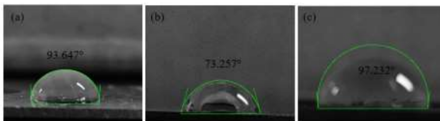
Figure 5.48: Surface wettability behaviour of (a) polished untreated Zn substrate, (b) Zn substrate after 7 hours of immersion in 1 M HCl medium with no inhibitor, and (c) in the presence of 800 ppm of ELJCE
