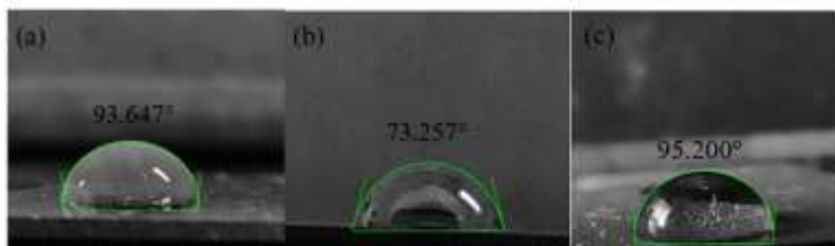
Figure 4.56: Surface wettability behaviour of (a) polished untreated Zn substrate, (b) Zn substrate after 7 hours of immersion in 1 M HCl medium with no inhibitor, and (c) in the presence of 800 ppm of MLJCE
