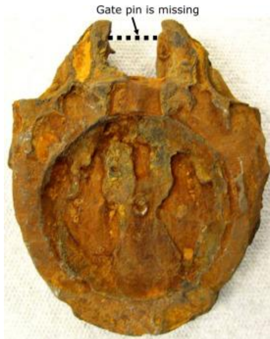
Figure 2.4: Corroded gate valve of a chemical transfer pipeline [57].
