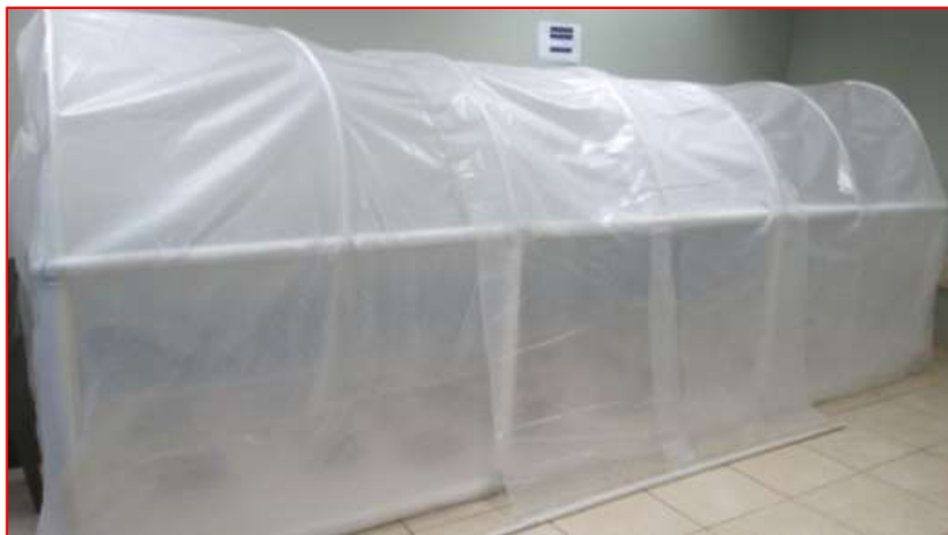
Fig.3.3 The healing chamber made of polyvinyl chloride which was used in the study.
