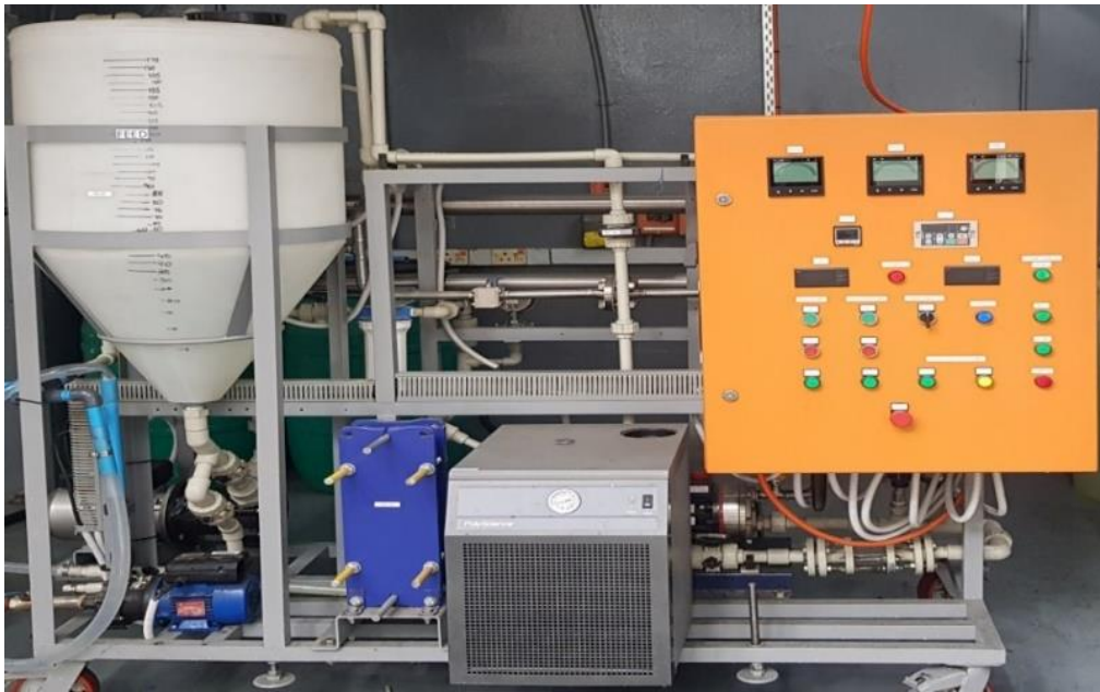
Figure 3.4: Pilot plant apparatus for membrane filtration processes
