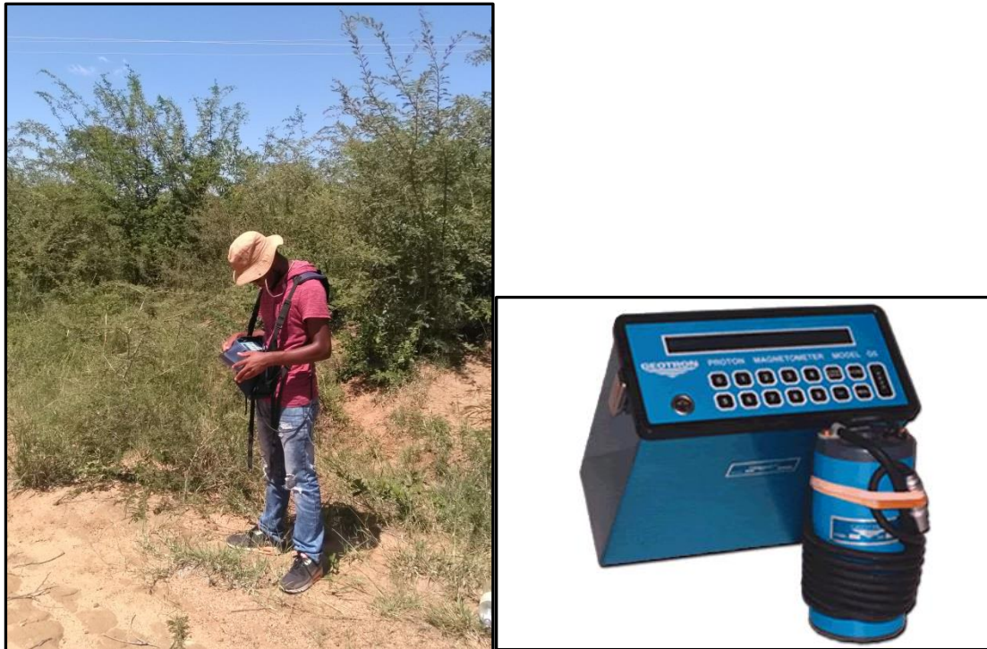
Figure 3.2: Geoproton (G5) Magnetometer
