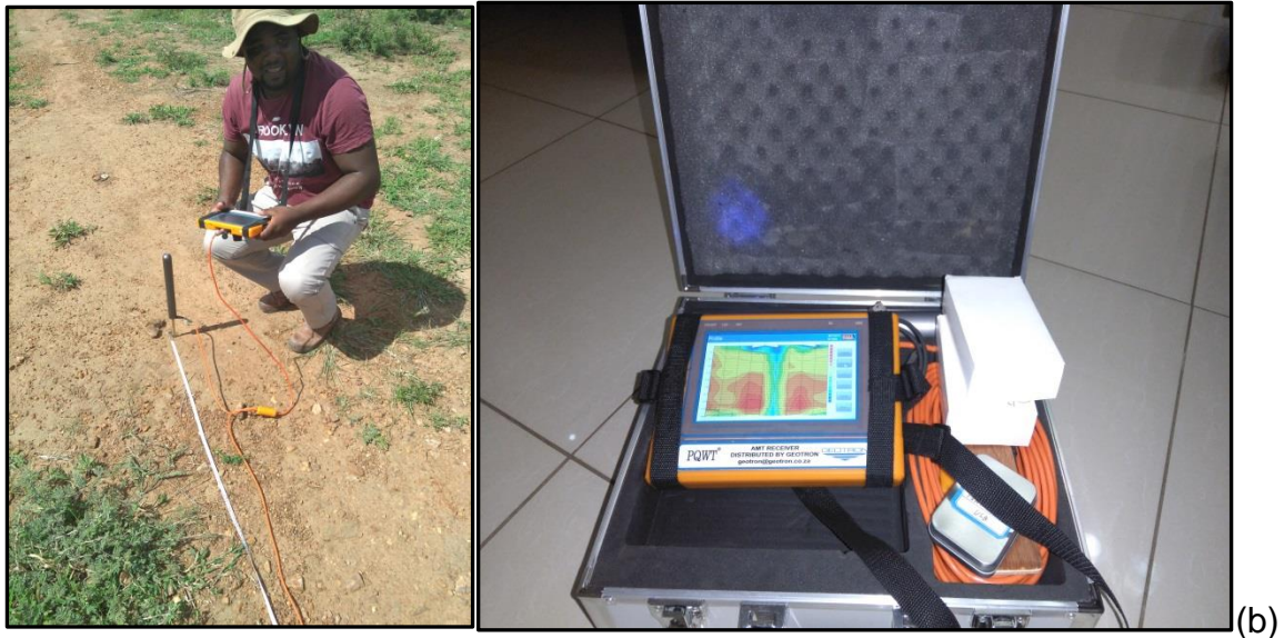
Figure 3.3: PQWTC-300 groundwater detector tool
