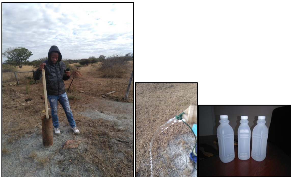
Figure 3.7: A bailer collecting water from the well into the sampling bottles
