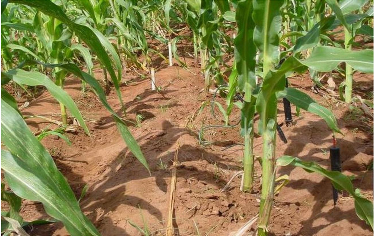
Figure 189: Wetting front detectors in one of the farmer's field
