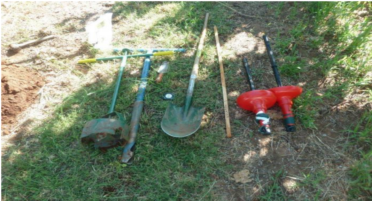
Figure 178: Tools used in preparation for the installation of Wetting Front Detectors
