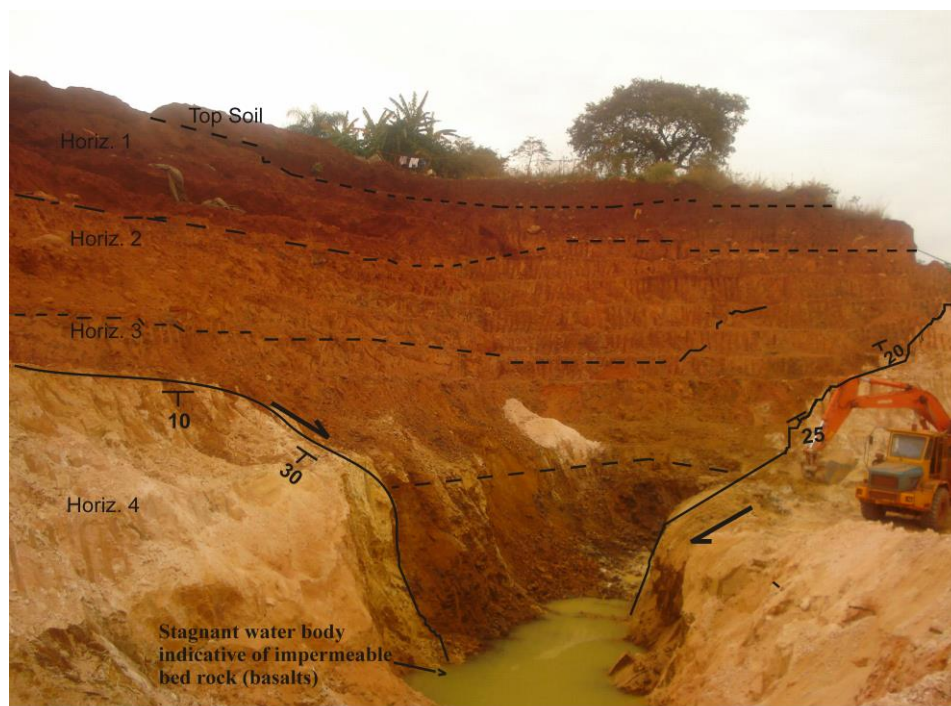
Figure 2.3 Partial view of Duthuni Kaolin quarry showing main horizons and structural controls.
