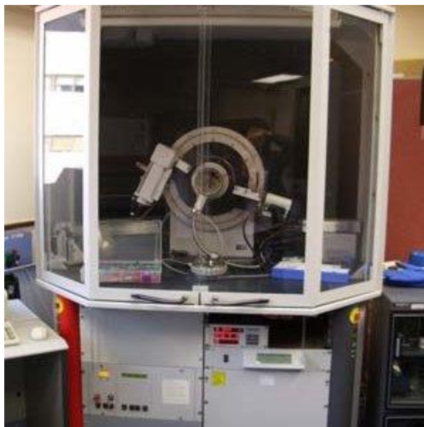
Figure 3.3: Bruker D8 Advance X-ray Diffractometer for mineral identification
