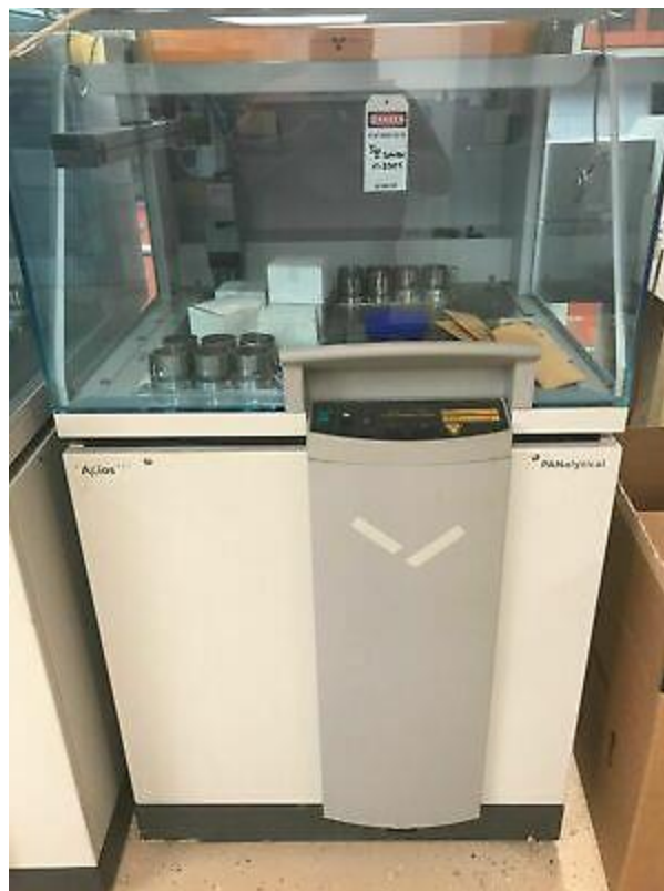
Figure 3.6: PANalytical Axios WDXRF spectrometer for elemental characterization
