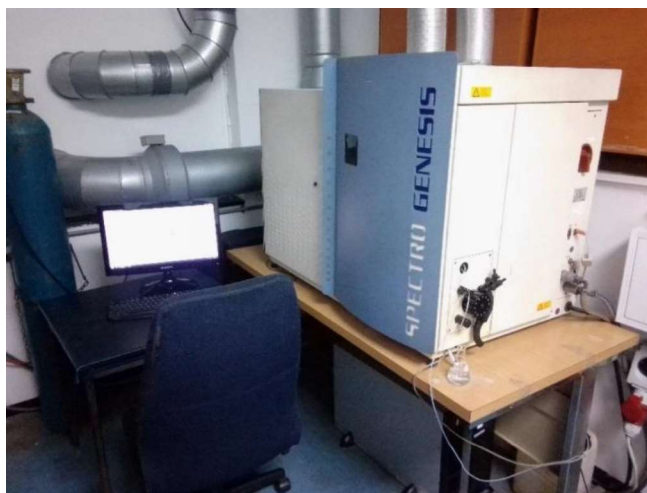
Figure 3.4: Inductively coupled plasma-optical emission spectroscopy (ICP - OES) laboratory set-up for the analysis
