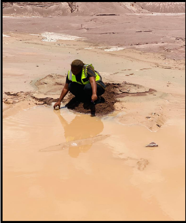
Figure 3.9: Water sampling at Zaaiplaats tin mine waste stagnant waters.
