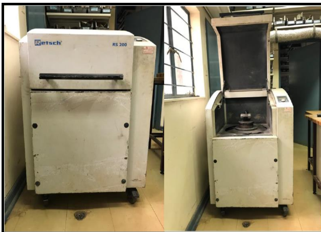
Figure 3.13: Restsch model RS 200 milling machine used to mill the samples.
