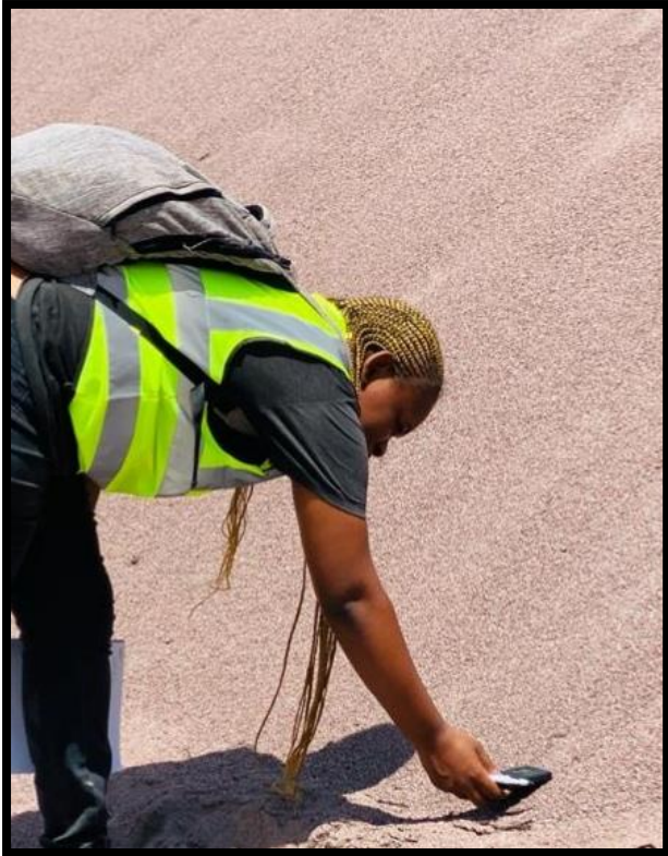
Figure 3.11: Radiation surveying using DP802i-RAYTECH Radiation Detector.
