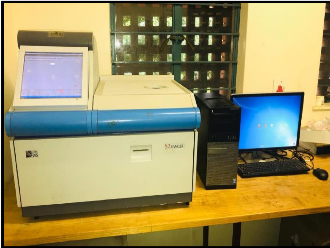
Figure 3.16: A Ranger S2 XRF Machine used for analysis.
