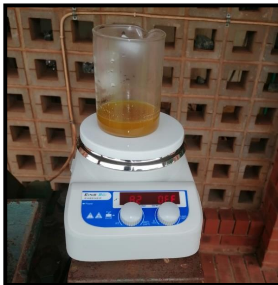
Figure 3.15: Digestion of plant samples using a hotplate.
