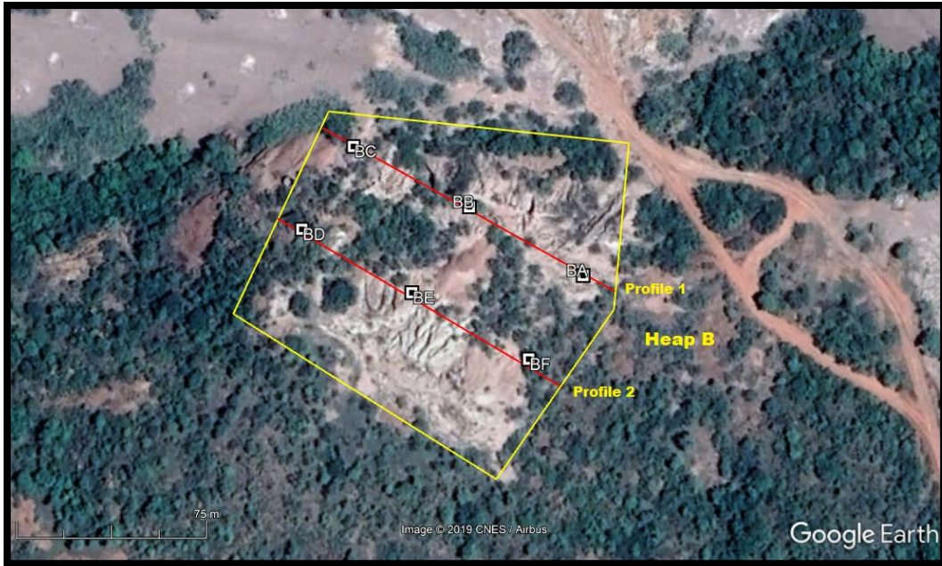
Figure 3.5: Sampling profiles and points in Heap B at Zaaiplaats tin mine.
