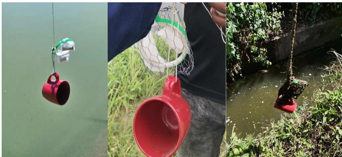
Figure 7. 3. SPATT samplers' configuration for field deployment
