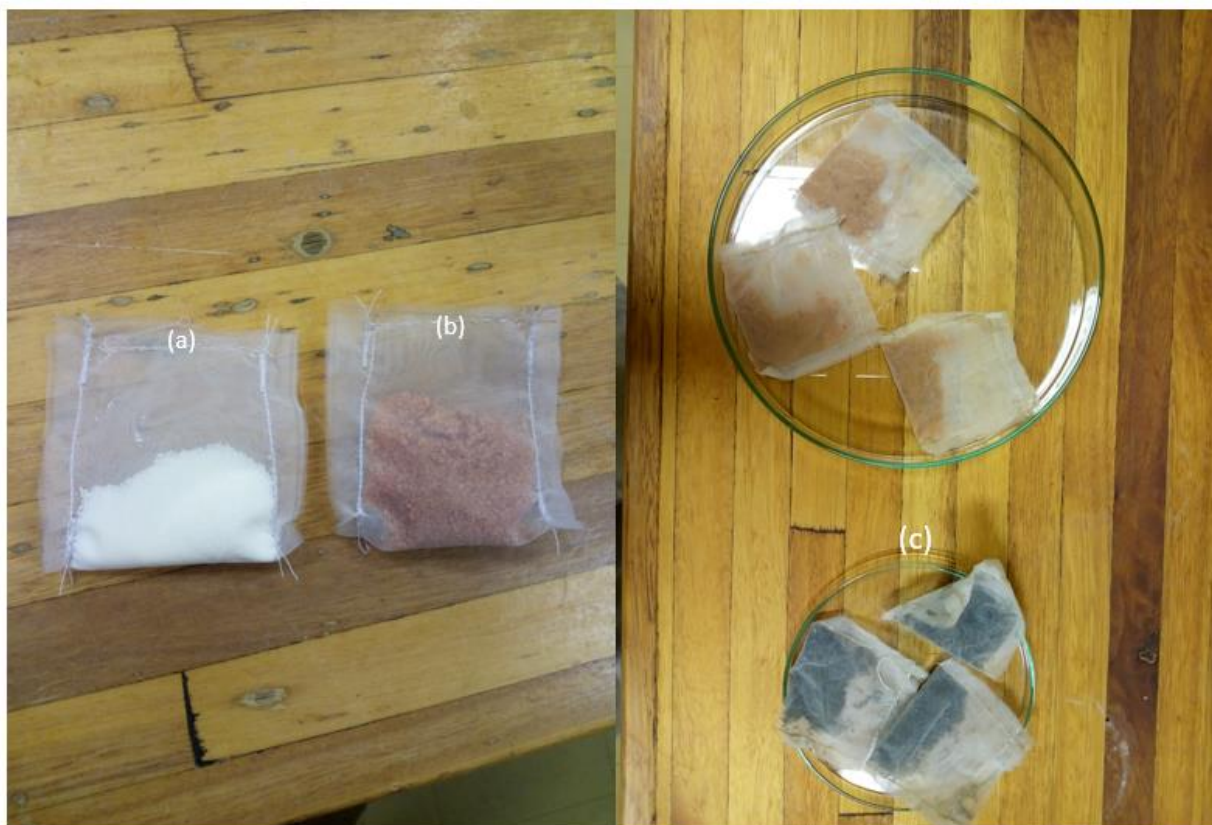
Figure 7. 1. Sorbents in SPATT bags (a) commercial DIAION HP20 (b) synthesized ChGLA (c) synthesized ChMWCNT
