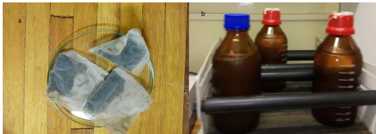
Figure 6. 1. (a) SPATT samplers packed with 0.2 g of the synthesized ChMWCNT composite (b) Laboratory adsorption experiment set-up with field water.
