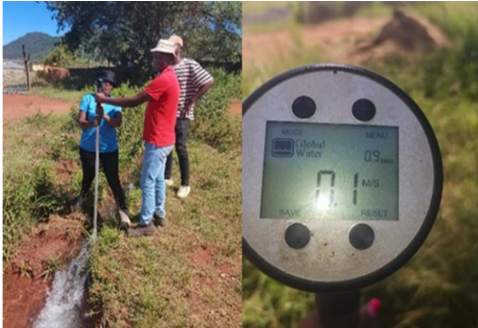
Figure 5: Measuring water flow velocity using global water flow meter
