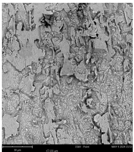
Figure 6.6: Scanning electron micrographs and EDS spectra of (a) freshly polished zinc (b) zinc 1.5 M HCl (c) zinc in 1.5 M HCl containing Chr-2-Carb.
