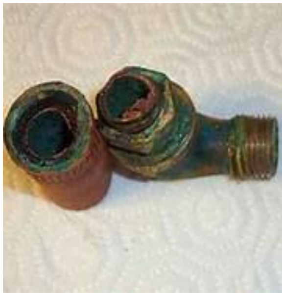
Figure 2.9: Dezincification as a result of selective corrosion.
