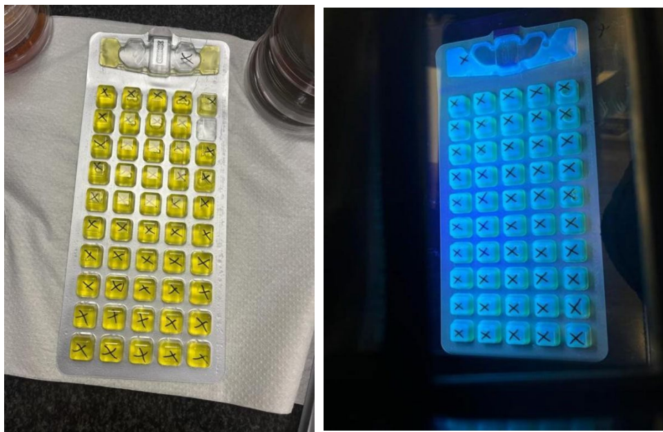
Figure 4.2: Detection of Total coliform and E. Coli: Colilert Q-Tray. Positive wells for total coliform (Left picture) and positive blue wells fluorescence for E. coli (right picture)
