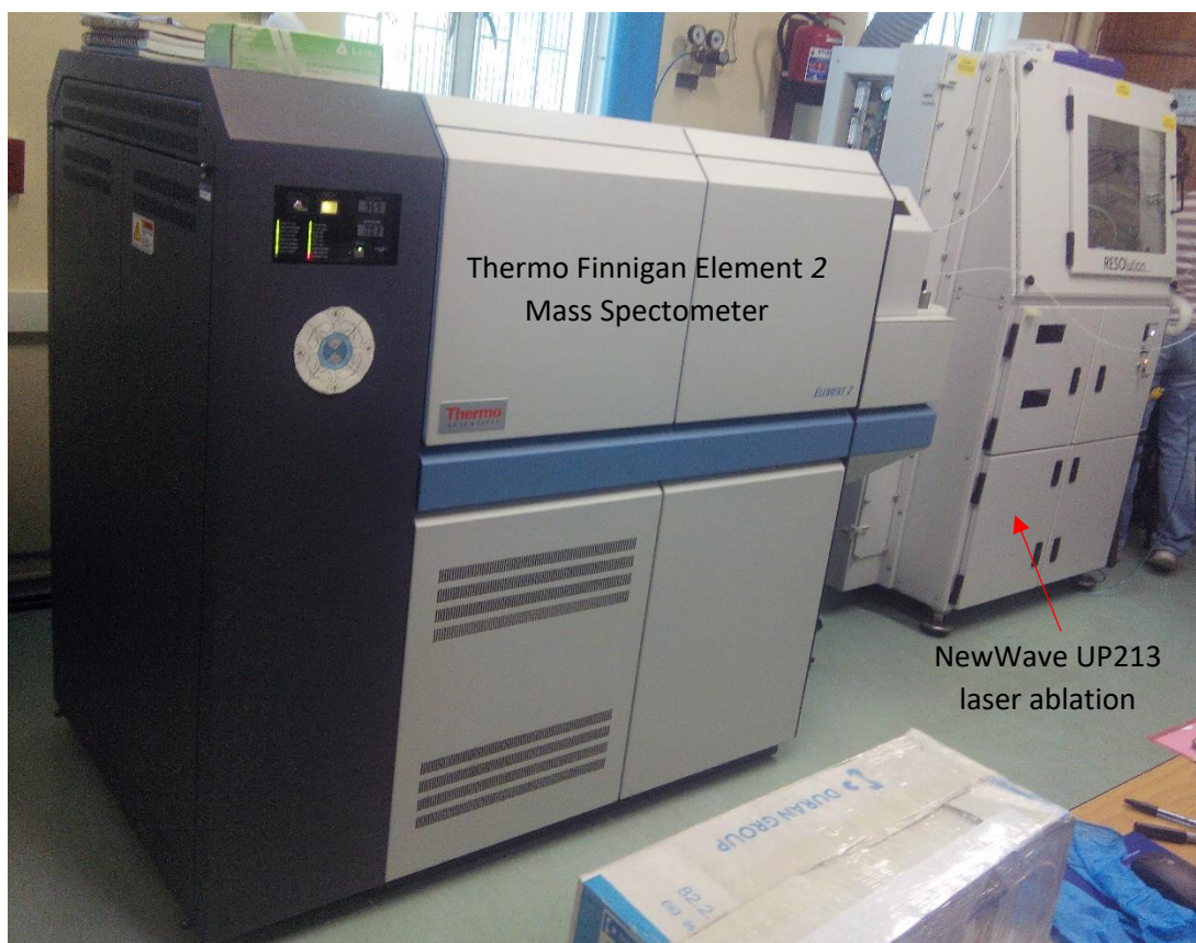
Figure 3.31: Laser ablation – single collector – magnetic sector field – inductively coupled plasma – mass spectrometer (LA-SFICP-MS) associated to a Thermo Finnigan Element 2 mass spectrometer coupled to a NewWave UP213 laser ablation system
