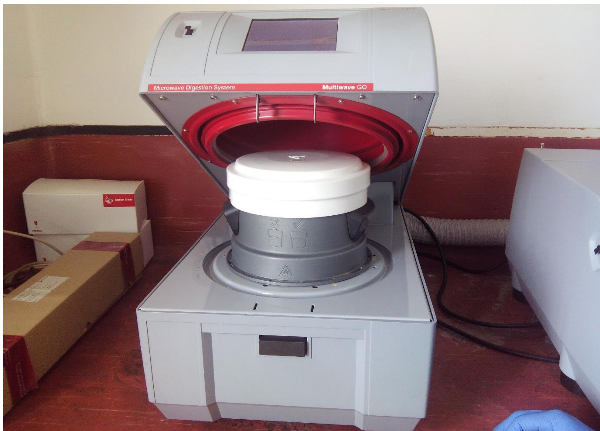
Figure 3.16: Multiwave GO Microwave Digestion System used to digest the samples
