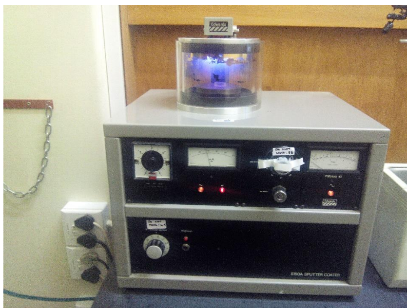
Figure 3.29: S150A sputter coater used for gold coating of mounts
