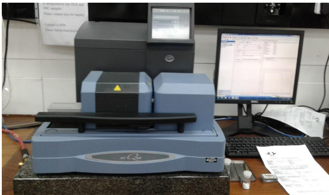
Figure 3.13: TA instrument SDT Q600 used for TGA-DSC analyses of samples
