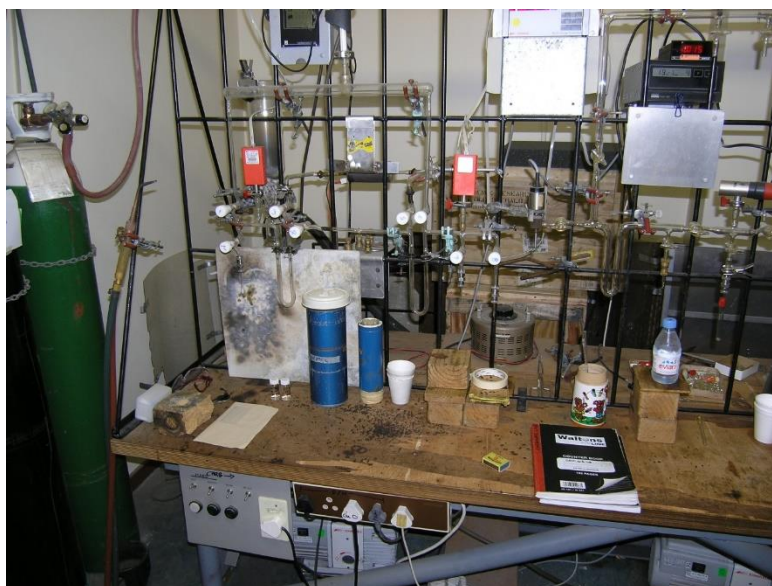
Figure 3.18: Set up for sample preparation for oxygen and hydrogen stable isotopes ratios
