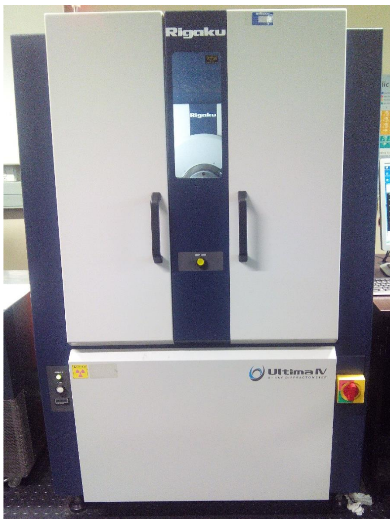
Figure 3.9: Rigaku Ultima IV X-ray diffractometer used for XRD analysis of samples
