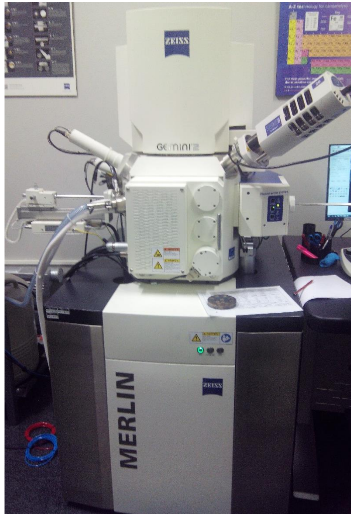
Figure 3.30: Zeiss MERLIN Field Emission Scanning Electron Microscope (FE-SEM) used for CL and BS imaging
