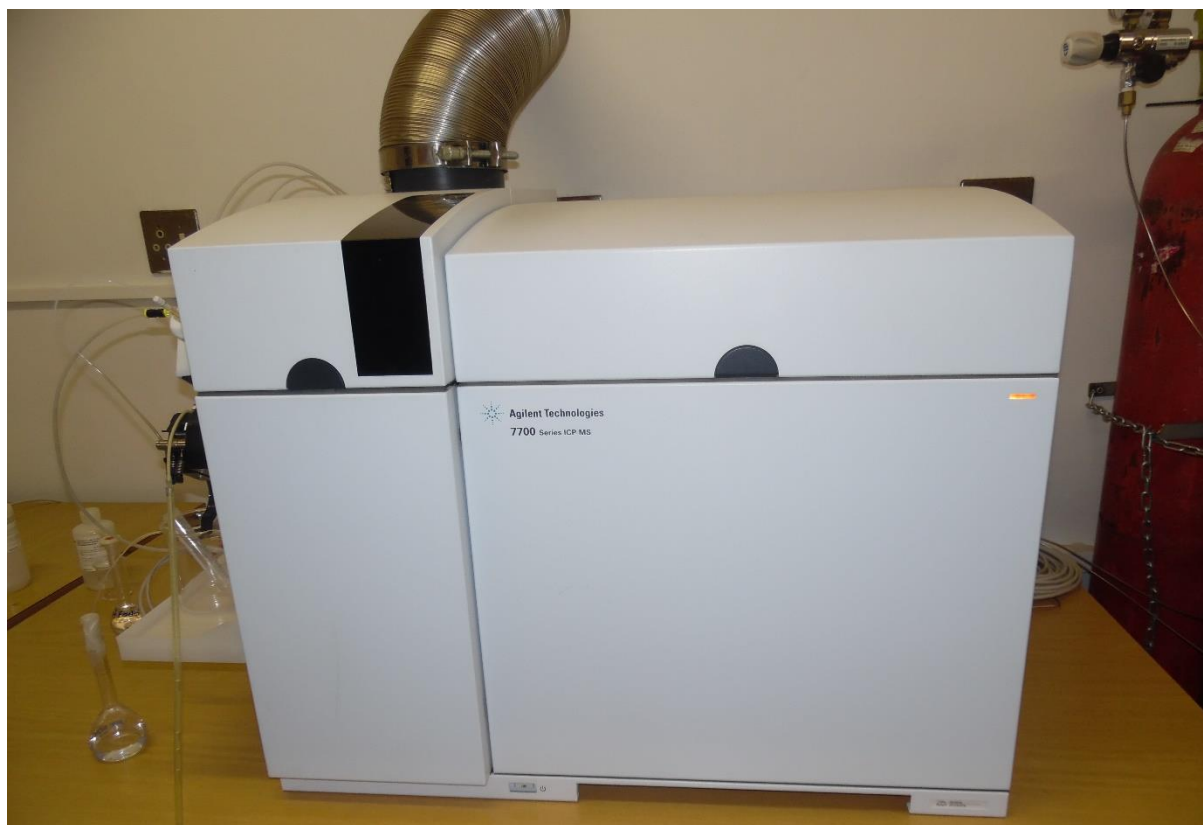
Figure 3.17: Agilent 7700 series ICP-MS spectrometer used for trace elements analysis
