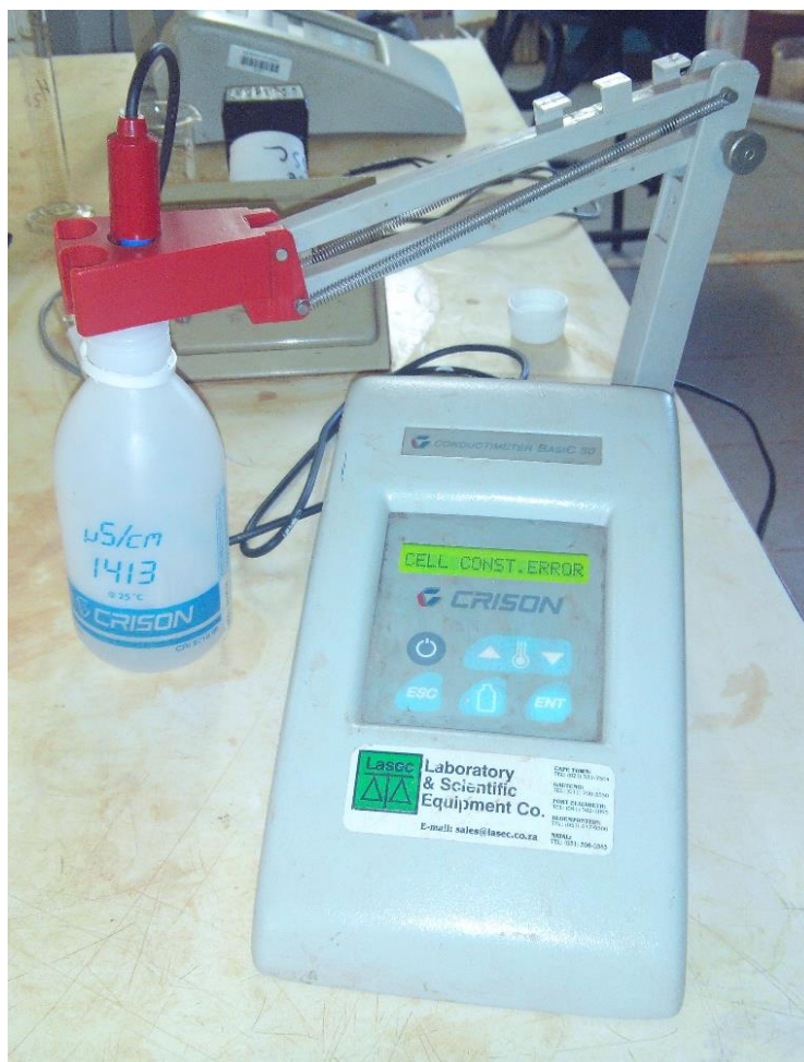
Figure 3.38: The Crison Basic 30 Conductimeter being calibrated
