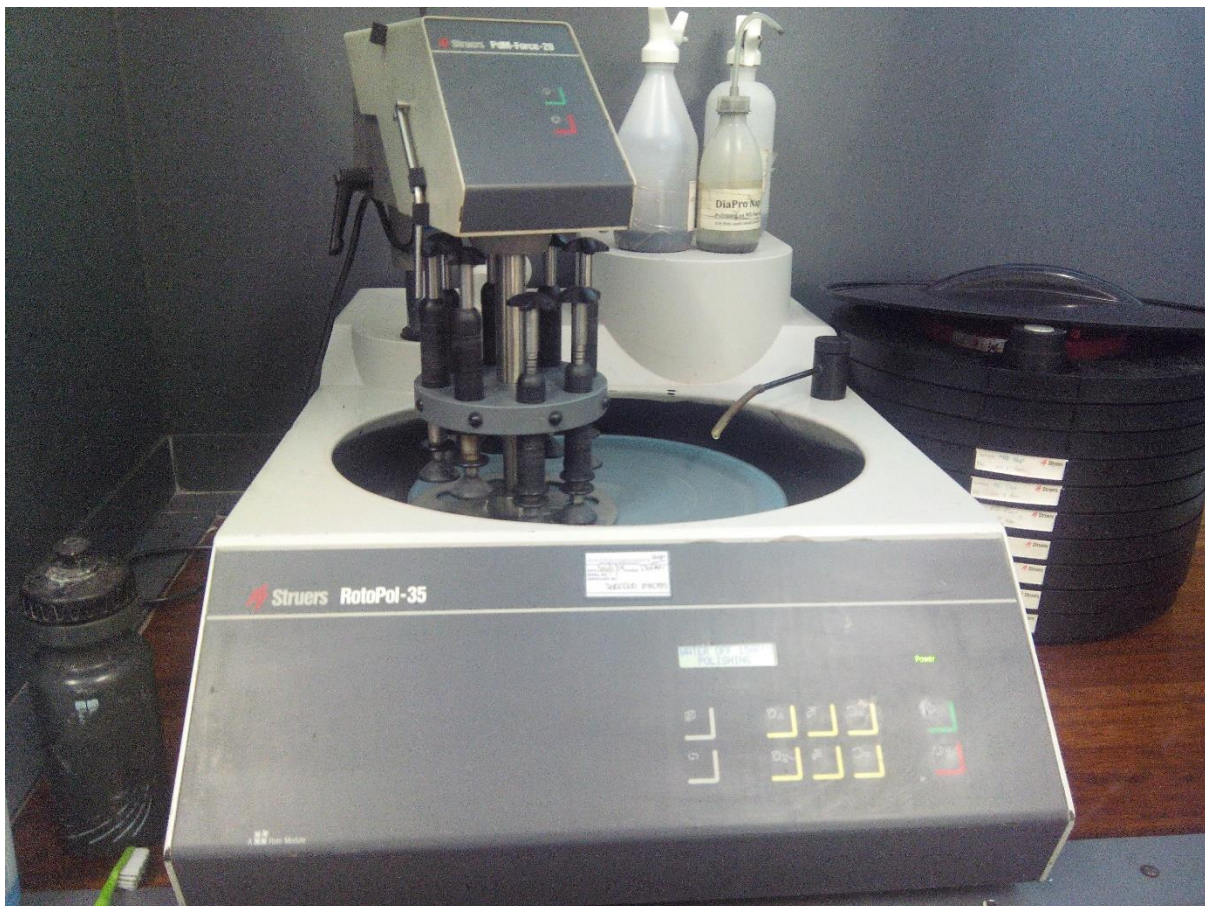
Figure 3.28: Struers Rotopol-35 used for mount polishing
