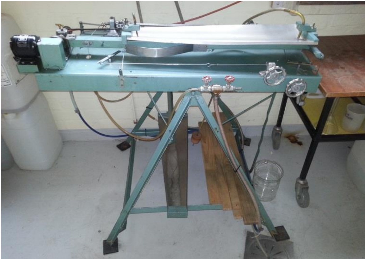
Figure 3.22: Super Panner used for separating heavy minerals from light minerals
