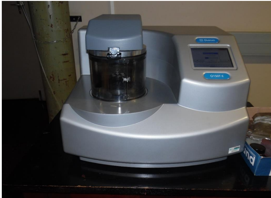
Figure 3.10: Quorum Q150T carbon coater, which was used to coat the samples
