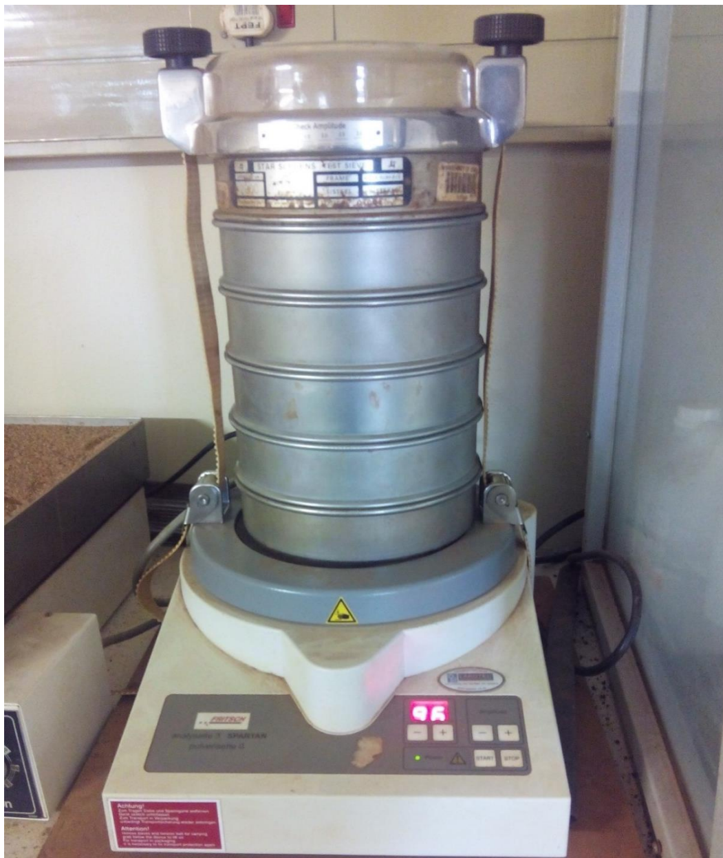
Figure 3.2: Nest of sieves comprising 2 mm, 1 mm, 125 \mu\text{m} , 105 \mu\text{m} , 63 \mu\text{m} sieves and the collection plate
