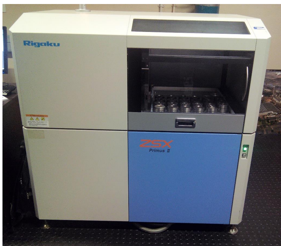
Figure 3.15: Rigaku ZSX Primus II XRF spectrometer used for XRF analysis of samples
