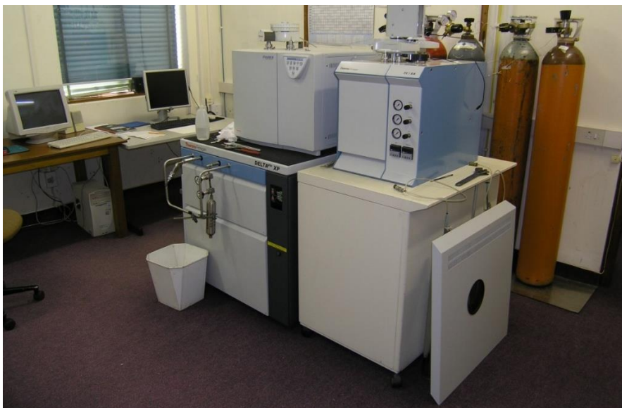
Figure 3.19: Finnegan DeltaXP mass spectrometer used for stable isotopes analyses
