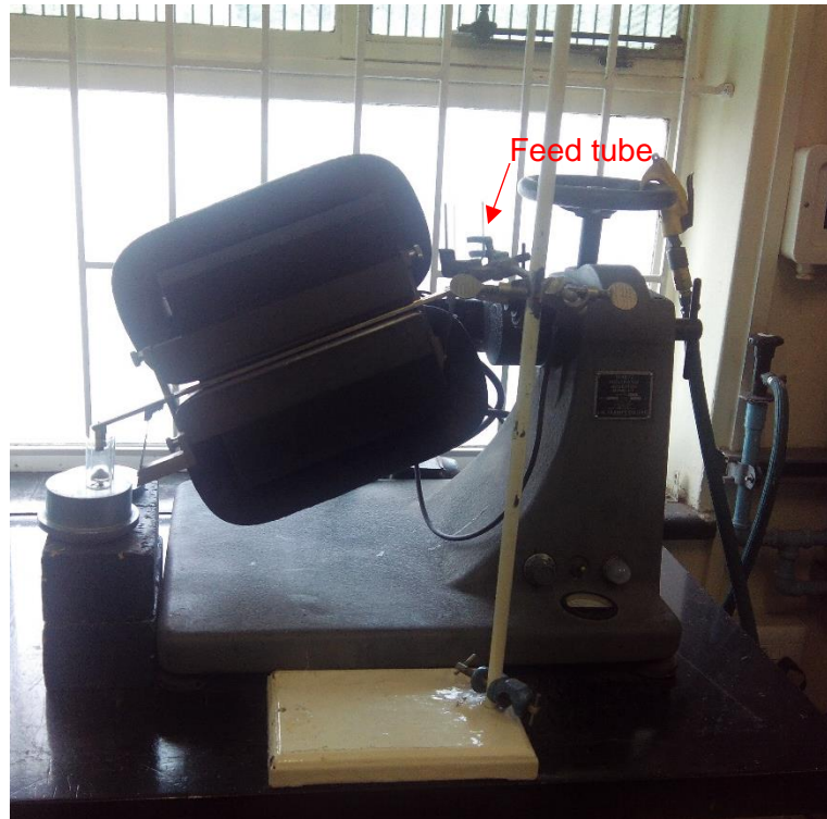
Figure 3.24: Franz magnetic separator used for separating paramagnetic minerals
