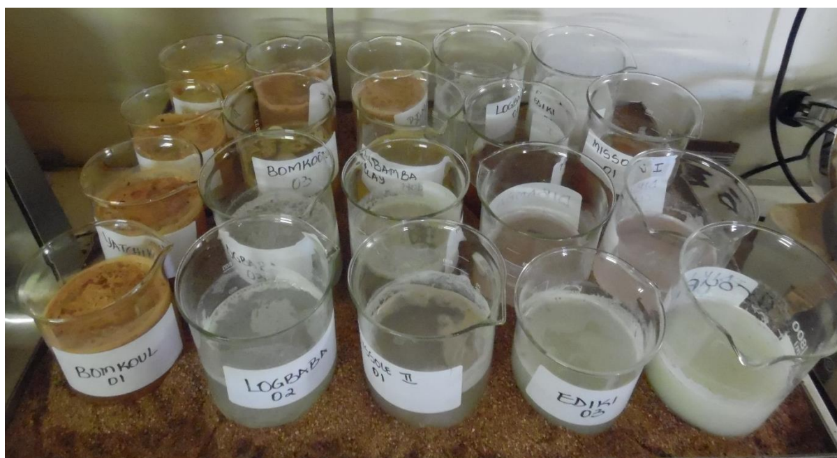
Figure 3.3: Samples being heated in a sand bath for oxidation of organic matter
