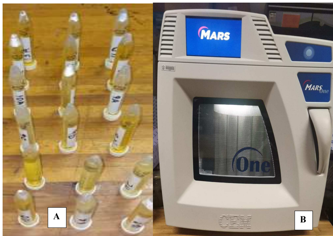
Figure 3. 3: Microwave Digestion used to digest water and sediments samples in this study. A- Digestate; B- MarsOne digester.
