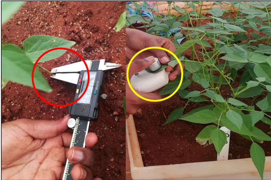
Fig. 3.3 The measuring of the stem diameter with a vernier caliper (red circle) and leaf chlorophyll content with a chlorophyll meter (yellow circle).
