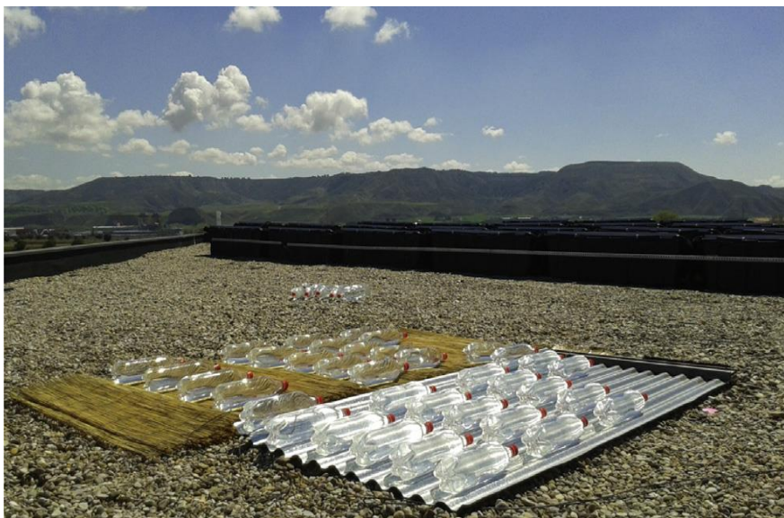
Figure 2.9: Experimental set-up of the solar disinfection tests (Vivar et al 2015)
