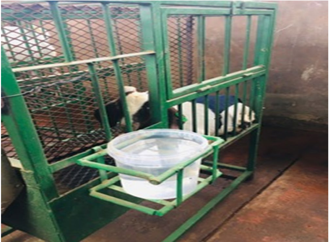
Figure 3.1: Metabolism cage/crate used for housing the goats
