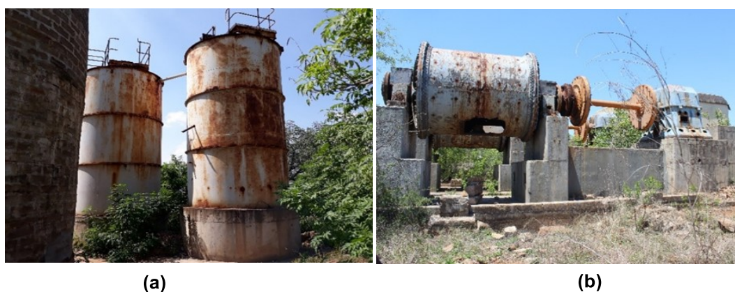
Figure 4. 8: Abandoned (a) agitation tanks and (b) ball mills at the mine sites
