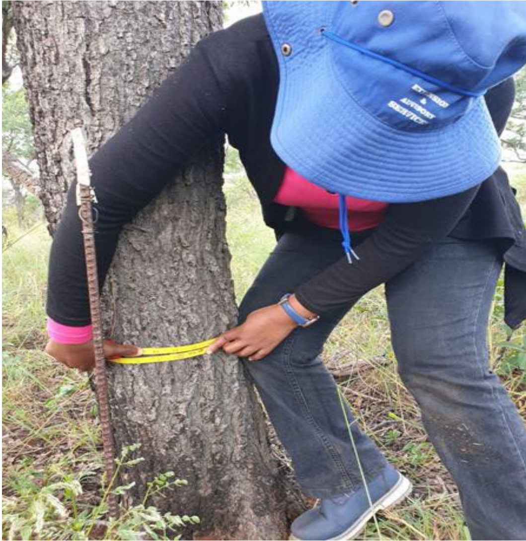
Figure 3.3: Measuring basal stem diameter using diameter tape.
