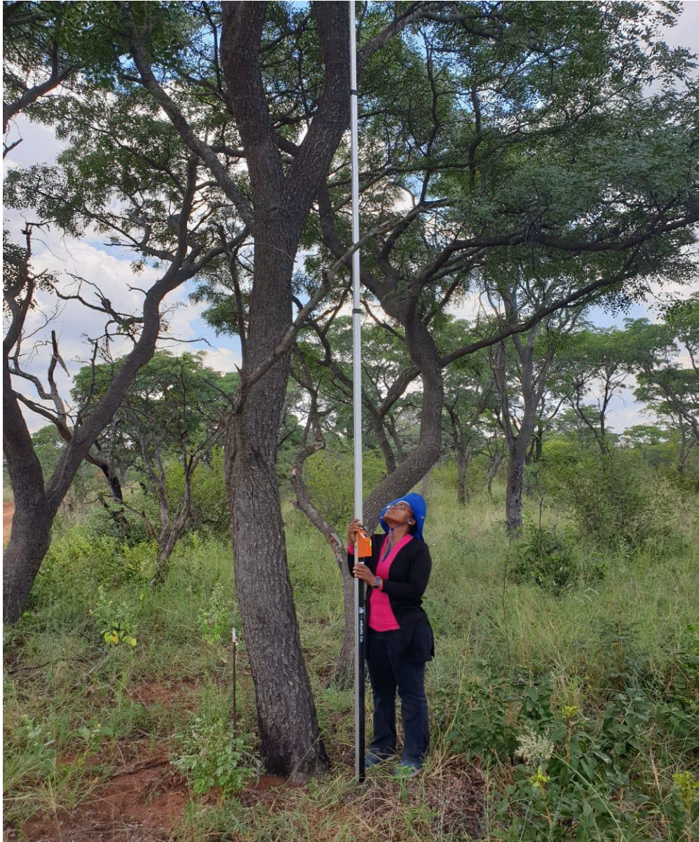
Figure 3.4: Measuring tree height using height meter rod.
