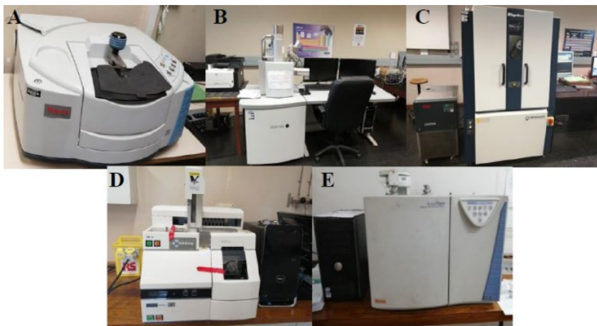
Figure 3.5. Equipment used for characterisation analysis includes FT-IR (A), SEM-EDX (B), XRD (C), TGA (D) and elemental analysis (E). (Picture taken by UJ lab technician Ms. N. Baloyi).
