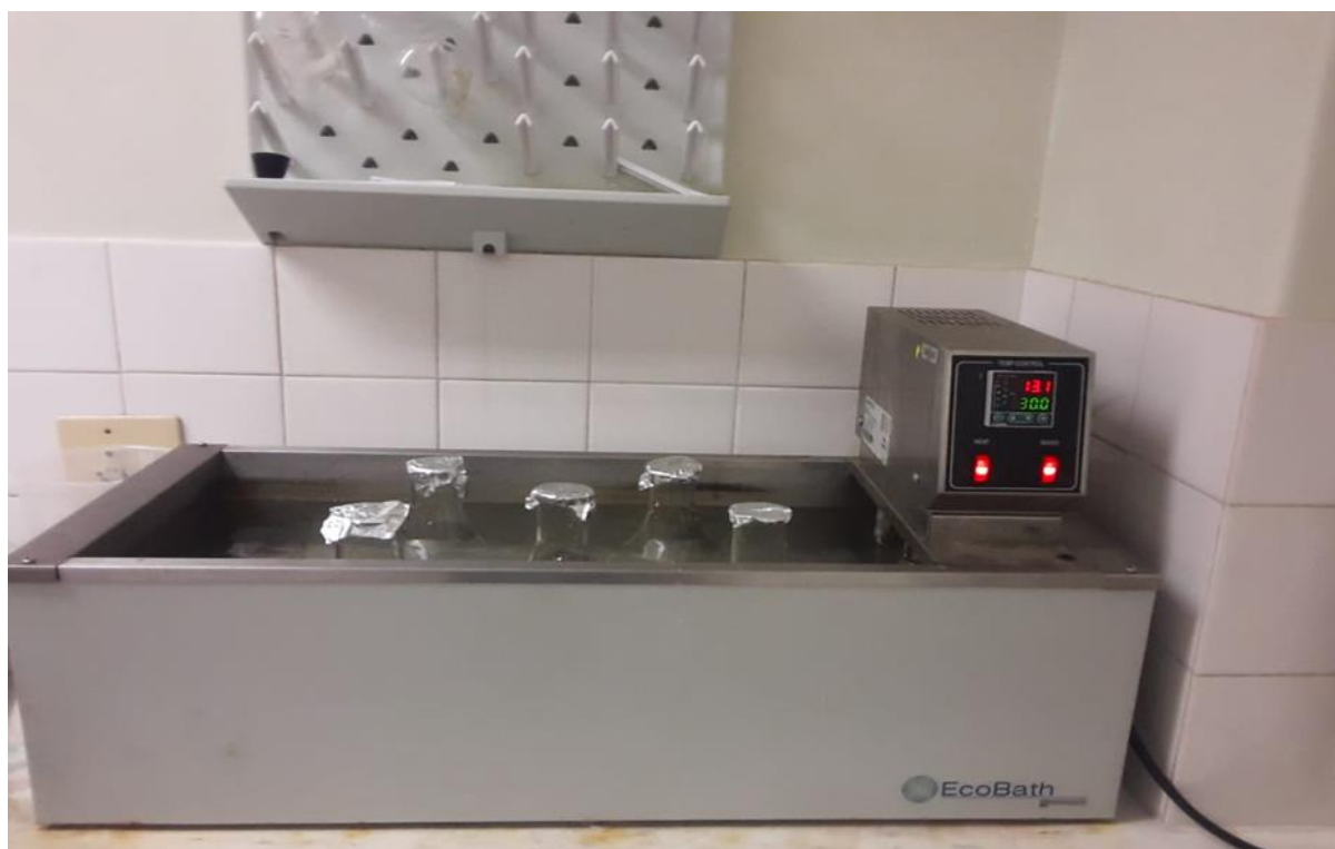
Appendix Figure A 1.0: Thermostatic water bath stirrer used for batch adsorption studies
