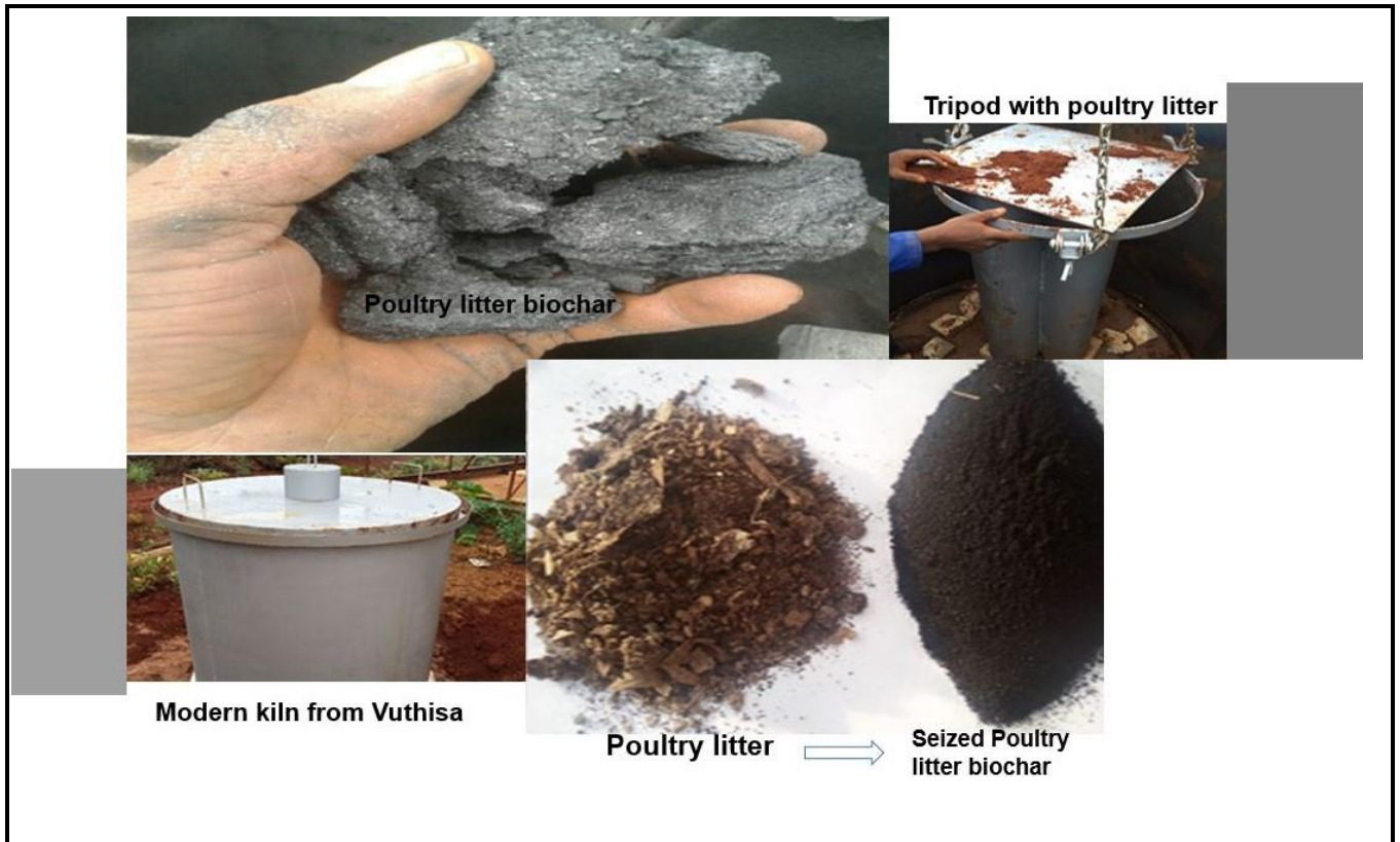
Picture A.1: Pyrolysis of poultry litter biochar using modern kiln from Vuthisa Pty, Ltd.
