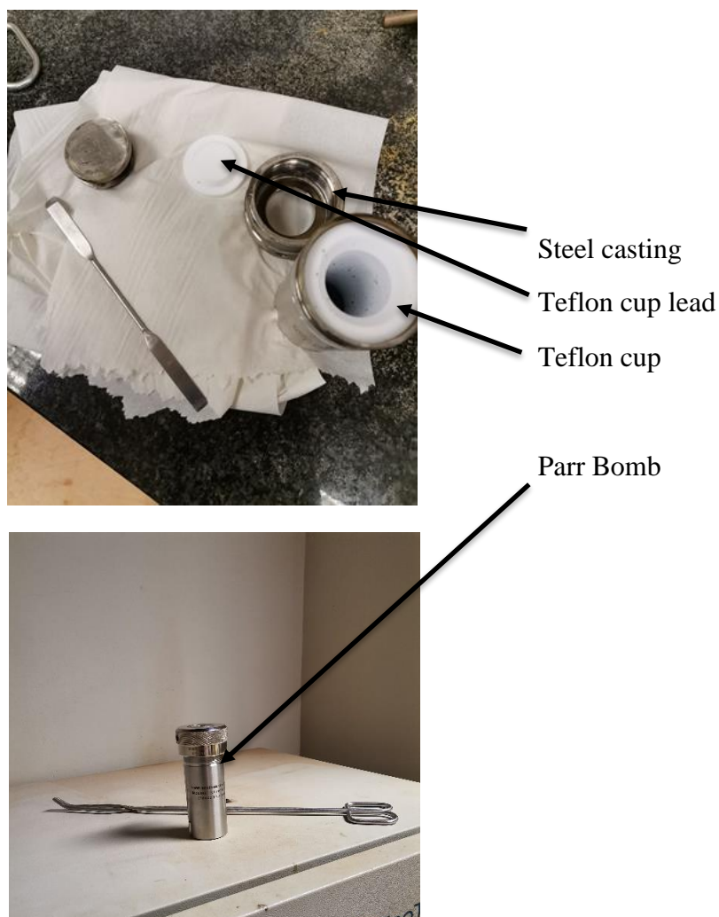
Fig 4: Parr bombs and Teflon lining used in the hydrothermal treatment process.
