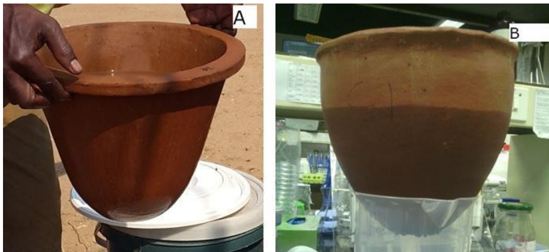
Fig. 8: Ceramic Water Filters (A) clay incorporated with silver nanoparticles from Mukondeni, Limpopo South Africa, (B) clay incorporated with sawdust from Sese, Zimbabwe. Adopted from Tshishonga and Gumbo (2017).
