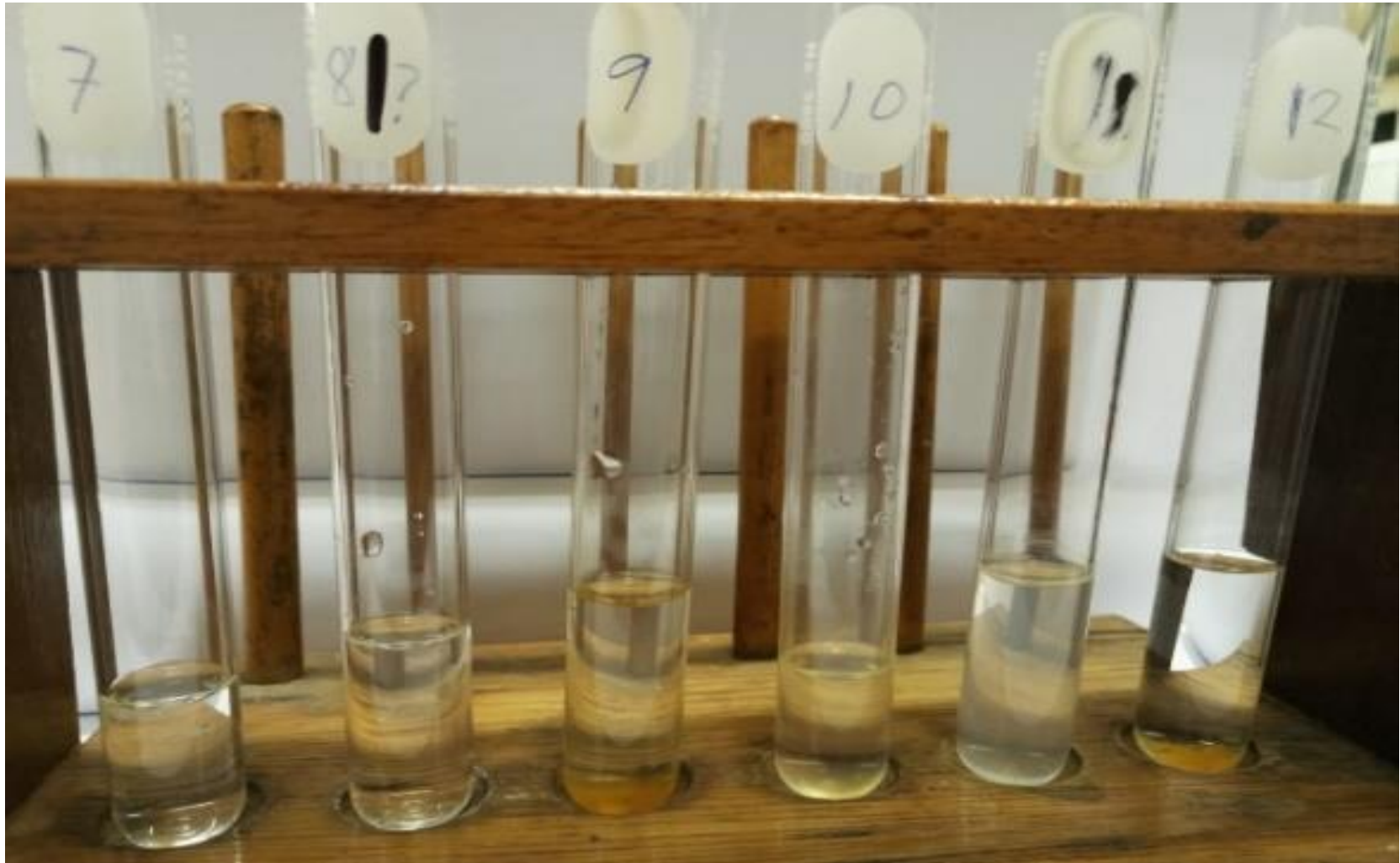
Figure 6. 4. Pictures of adsorbent treated synthetic oily wastewater (Experimental conditions are as presented in columns 1 to 3 of Table 6.3).
