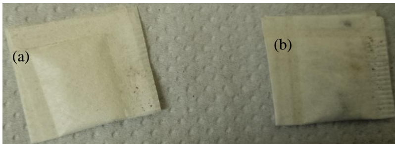
Figure 4. 1. (a) sealed empty tea bag (b) sealed tea bag containing adsorbents.
