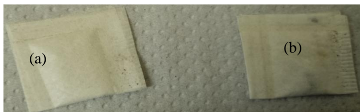
Figure 6. 1. (a) sealed empty tea bag (b) sealed tea bag containing adsorbents.
