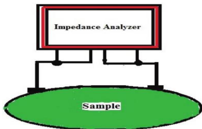
Figure 4.9. Two-electrode impedance measurement technique [13].
