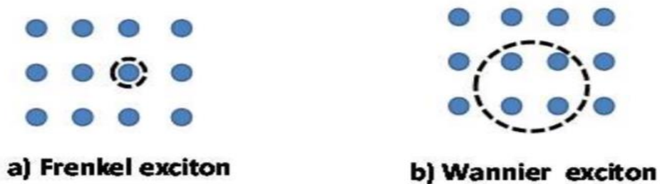
Figure 3.18 a) Frenkel exciton and b) Wannier exciton typified by dashed circles (shaded circles symbolize atoms or molecules).
