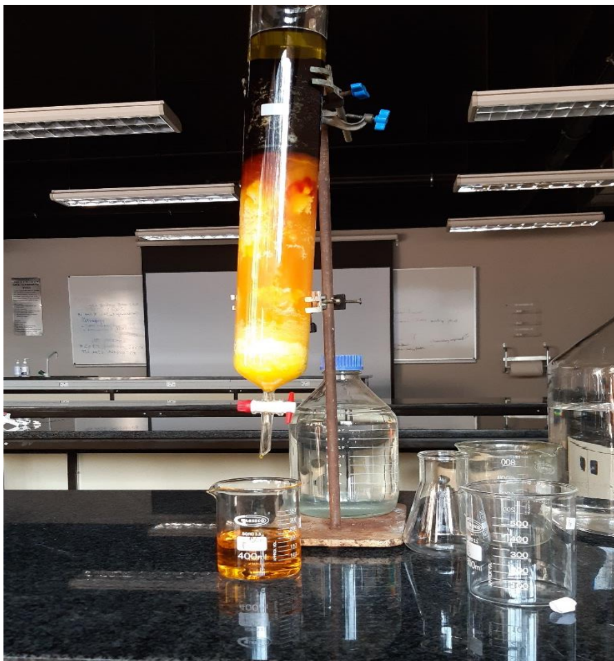
Figure 4.3: Column chromatography the second fraction collection of DCM crude extract F2 eluted by DCM 100%
